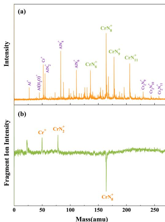
Fig. 1 (a) Mass spectra of CrN<sub>n</sub><sup>0/+</sup> clusters produced by laser bombardment of Cr/AlN samples. (b) Photolysis mass spectra of CrN<sub>8</sub><sup>+</sup> cluster at 266 nm.
