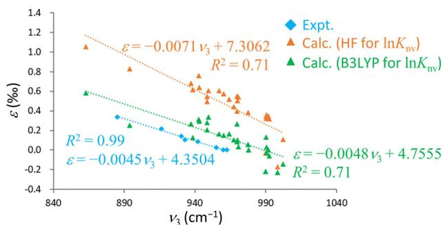
**Fig. 4** Relationships between  $\nu_3$  and  $\epsilon$ . The horizontal axis shows  $\nu_3$  in units of  $\text{cm}^{-1}$  while the vertical axis shows  $\epsilon$  in units of ‰. The dotted lines are linear regressions and  $r^2$  is the coefficient of determination in each case.
