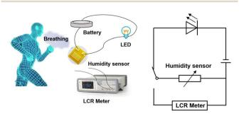
Fig. 2 Circuit diagram for the humidity sensor system for monitoring breathing (LED) and ambient humidity (LCR)
