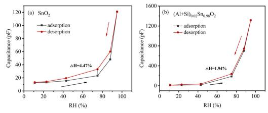
Fig. 12 Humidity hysteresis characteristics of (a) pure SnO<sub>2</sub> and (b) (Al + Si)<sub>0.02</sub>Sn<sub>0.98</sub>O<sub>2</sub> humidity sensors.
