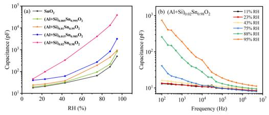
Fig. 11 (a) Capacitance relative humidity curves of pure and Al-Si co-doped SnO<sub>2</sub> humidity sensors. (b) Capacitance frequency curves of (Al +  $Si)_{0.02}Sn_{0.98}O_2$  in different RH
