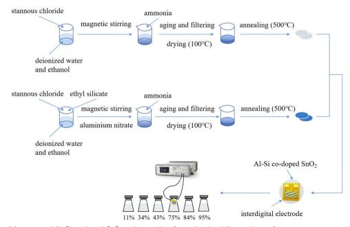
Fig. 1 Preparation of the pure and Al-Si co-doped SnO<sub>2</sub> and procedure for testing humidity sensing performance.
