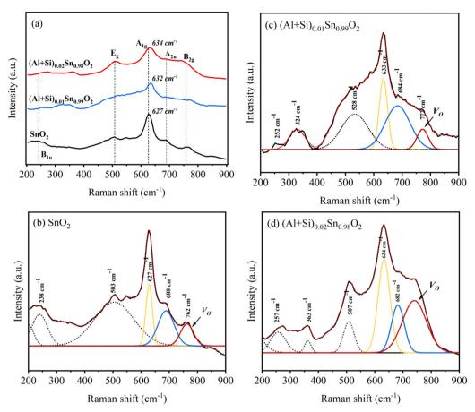
Raman spectra of pure and Al-Si co-doped SnO<sub>2</sub> (a) general survey spectrum, (b)-(d) deconvolution of the Raman spectrum.
