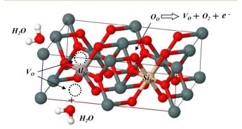
Fig. 15 Structure diagram of the defects  $Al_{Sn} + Si_{Sn} + V_O$  reacting with water molecules
