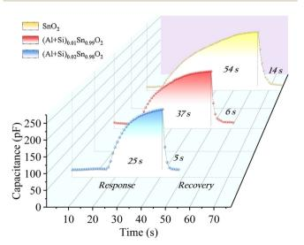
Fig. 13 Response/recovery time of pure and Al-Si co-doped SnO<sub>2</sub> humidity sensors at the humidity ranging from 11% to 95% RH.
