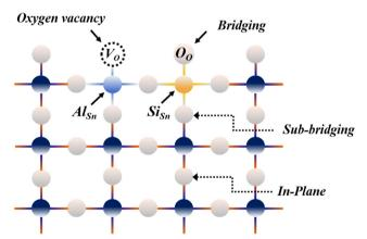
Fig. 6 The illustration of different modes of oxygen atoms on the SnO<sub>2</sub> surface
