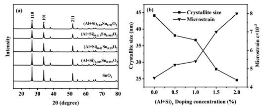
Fig. 3 (a) X-ray diffraction patterns of pure and Al-Si co-doped SnO<sub>2</sub>. (b) Plots of crystallite size and microstrain versus doping concentrations of (Al +  $Si)_x Sn_{(1-x)}O_2$
