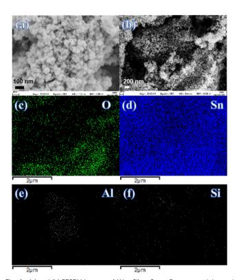
Fig. 4 (a) and (b) FESEM images of (Al + Si)<sub>0.02</sub>Sn<sub>0.98</sub>O<sub>2</sub> nanoparticles and (c)-(f) (Al + Si) elemental mapping images.
