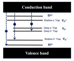
Fig. 10 A schematic band diagram with defect states.
