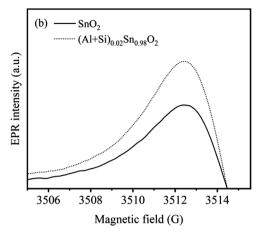
Fig. 7 (a) and (b) EPR spectrum and intensity comparison of pure  $SnO_2$  and  $(Al + Si)_{0.02}Sn_{0.98}O_2$
