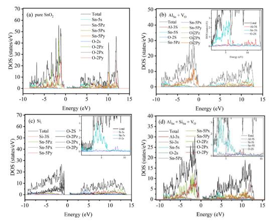
TDOS and PDOS for (a) pure  $SnO_2$ , (b)  $Al_{Sn} + V_O$ , (c)  $Si_i$  and (d)  $Al_{Sn} + Si_{Sn} + V_O$
