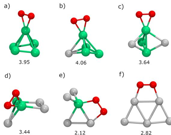
Fig. 4 The most stable structures for  $\text{O}_2$  adsorption on gas-phase  $\text{Re}_n\text{Pt}_m$  ( $n + m = 5$ ) clusters: (a)  $\text{Re}_5$ , (b)  $\text{Re}_4\text{Pt}_1$ , (c)  $\text{Re}_3\text{Pt}_2$ , (d)  $\text{Re}_2\text{Pt}_3$ , (e)  $\text{Re}_1\text{Pt}_4$ , (f)  $\text{Pt}_5$ . The adsorption energy ( $E_{\text{ads}}$ ) is displayed below each structure in eV.
