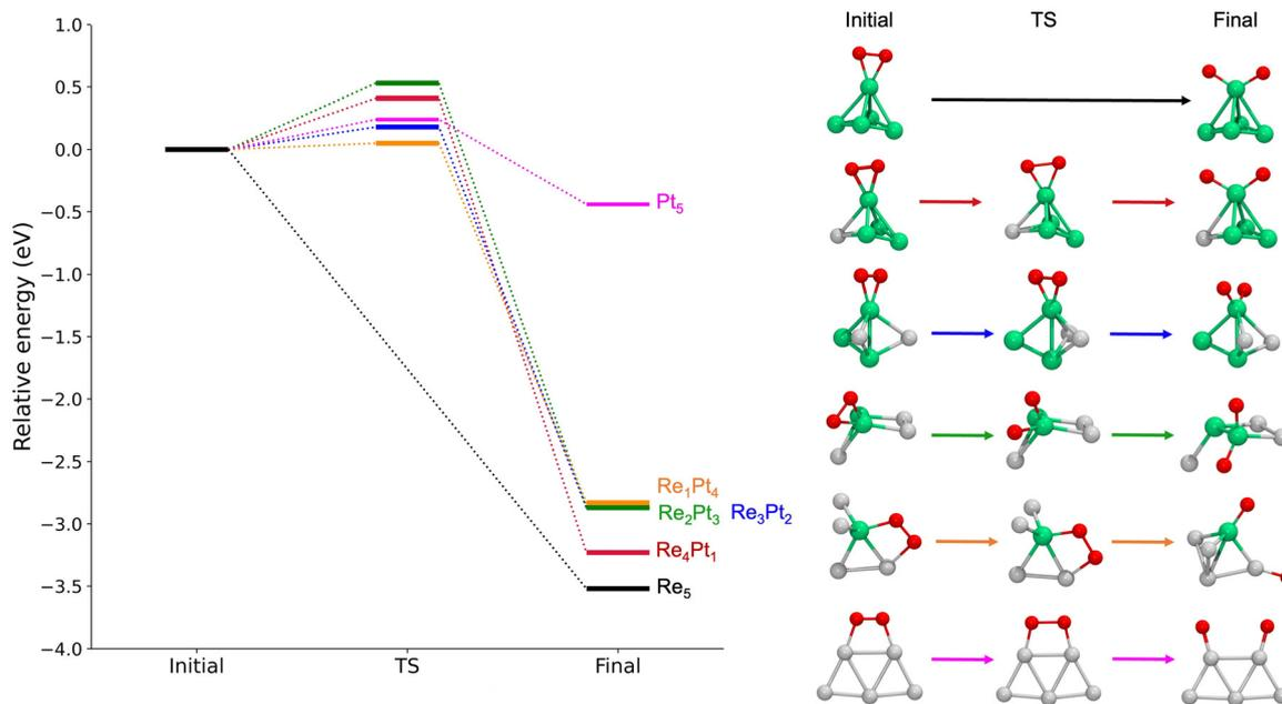
Fig. 7 Left panel: Reaction energetics for the dissociation of O<sub>2</sub> on gas-phase Re<sub>7</sub>Pt<sub>m</sub> clusters. All the energies are shown relative to the one of the initial state, on each case. Right panel: Structures for initial, transition and final states for each cluster. The colors of the atoms are consistent with those in previous figures.
