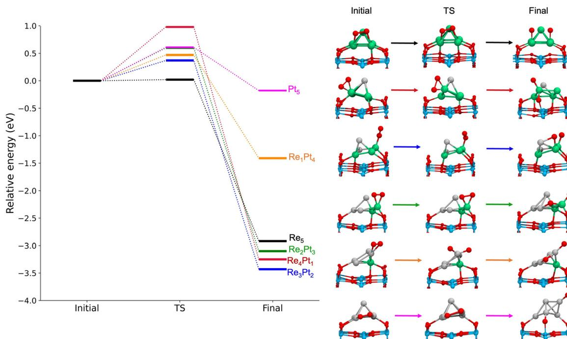
Fig. 8 Left panel: Reaction energetics for the dissociation of O<sub>2</sub> on supported Re<sub>7</sub>Pt<sub>m</sub> clusters. All the energies are shown relative to the one of the initial state, on each case. Right panel: Structures for initial, transition and final states for each cluster. The colors of the atoms are consistent with those in previous figures.
