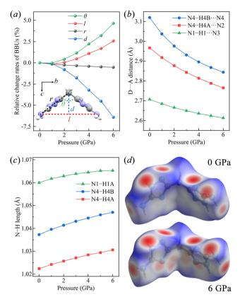
Fig. 3 (a) Relative change rates of BBUs as a function of pressure from 0 to 6 GPa. Evolution of the (b) D...A distance of hydrogen bonds and (c) N-H length as a function of pressure. (d) Hirshfeld surface of BATZM at ambient pressure (top) and 6 GPa (bottom). All data are calculated using the DFT-D3(BJ) dispersion correction.
