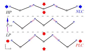
Fig. 4 Schematic of the mechanism of the abnormal mechanical behavior along the b-axis of the BATZM crystal.
