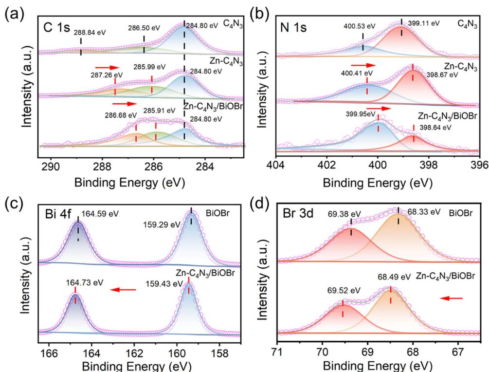
Fig. 2 C 1s (a), N 1s (b), Bi 4f (c) and Br 3d (d) XPS spectra of C<sub>4</sub>N<sub>3</sub>, Zn-C<sub>4</sub>N<sub>3</sub>, BiOBr and Zn-C<sub>4</sub>N<sub>3</sub>/BiOBr.
