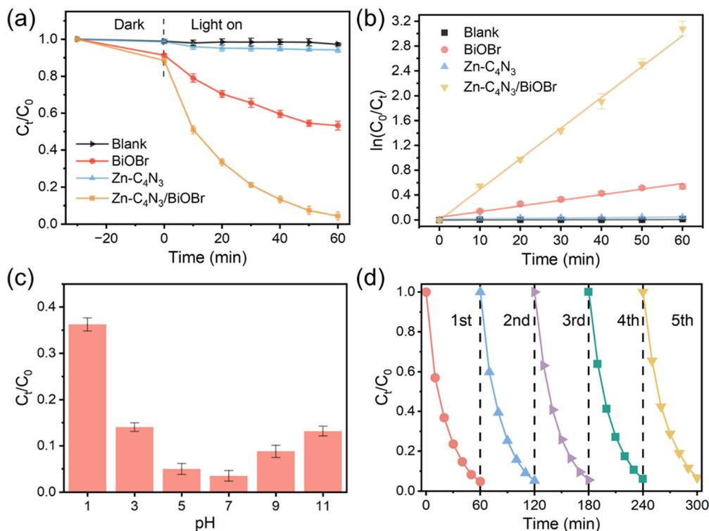
Fig. 5 (a) Photodegradation of TC at photocatalysts. (b) Degradation reaction kinetics of TC over photocatalysts. (c) Effect of the initial pH value over Zn-C<sub>4</sub>N<sub>3</sub>/BiOBr in degradation of TC. (d) Five recycling runs over Zn-C<sub>4</sub>N<sub>3</sub>/BiOBr in degradation of TC. Note that the experiment in Fig. 5a was conducted without pH adjustment.
