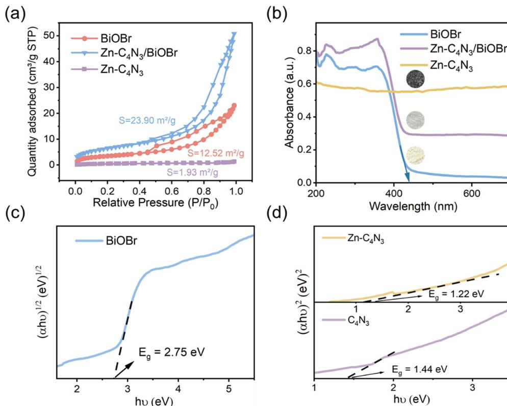
Fig. 3 (a) N<sub>2</sub> adsorption–desorption isotherms of BiOBr and  $Zn-C_4N_3/BiOBr$ . (b) UV-vis absorption spectra of the different catalysts (inset: digital pictures of photocatalysts). (c) and (d) The band gaps of BiOBr,  $C_4N_3$  and  $Zn-C_4N_3$ .
