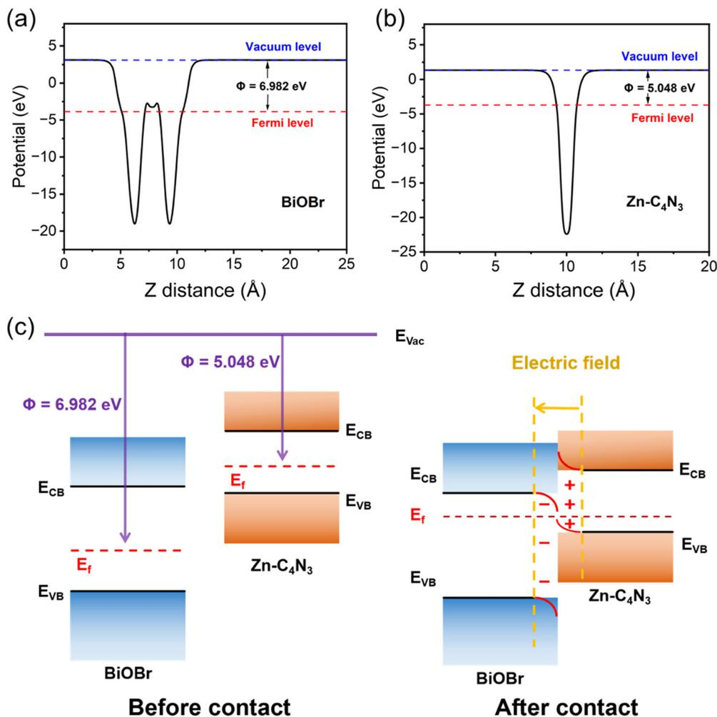
Fig. 6 The work function of (a) BiOBr and (b) Zn-C<sub>4</sub>N<sub>3</sub>. (c) Schematic illustration of the Zn-C<sub>4</sub>N<sub>3</sub>/BiOBr heterostructure: before and after contact in the dark.
