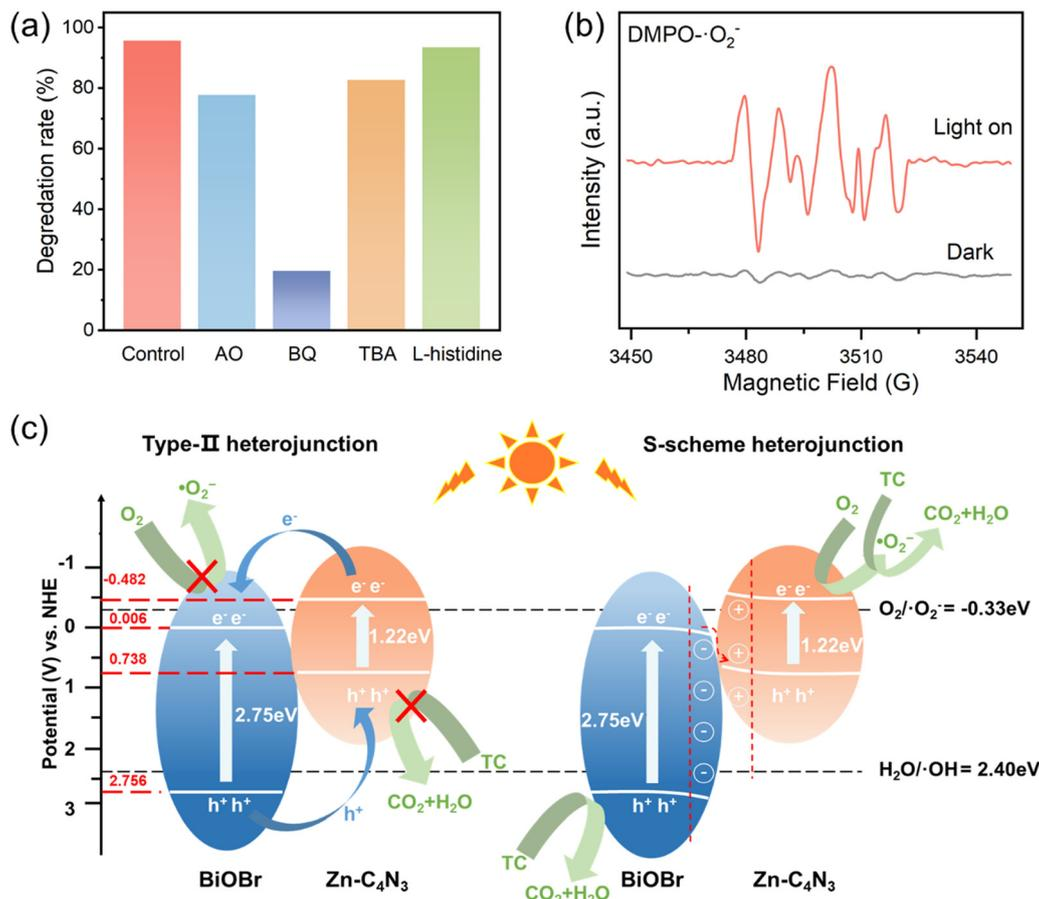
Fig. 7 (a) Trapping experiments of active species about the photocatalytic degradation of TC. (b) ESR spectra of DMPO- $\cdot\text{O}_2^-$  in methanol dispersions over Zn-C<sub>4</sub>N<sub>3</sub>/BiOBr after irradiation. (c) Possible photocatalytic mechanism for Zn-C<sub>4</sub>N<sub>3</sub>/BiOBr.
