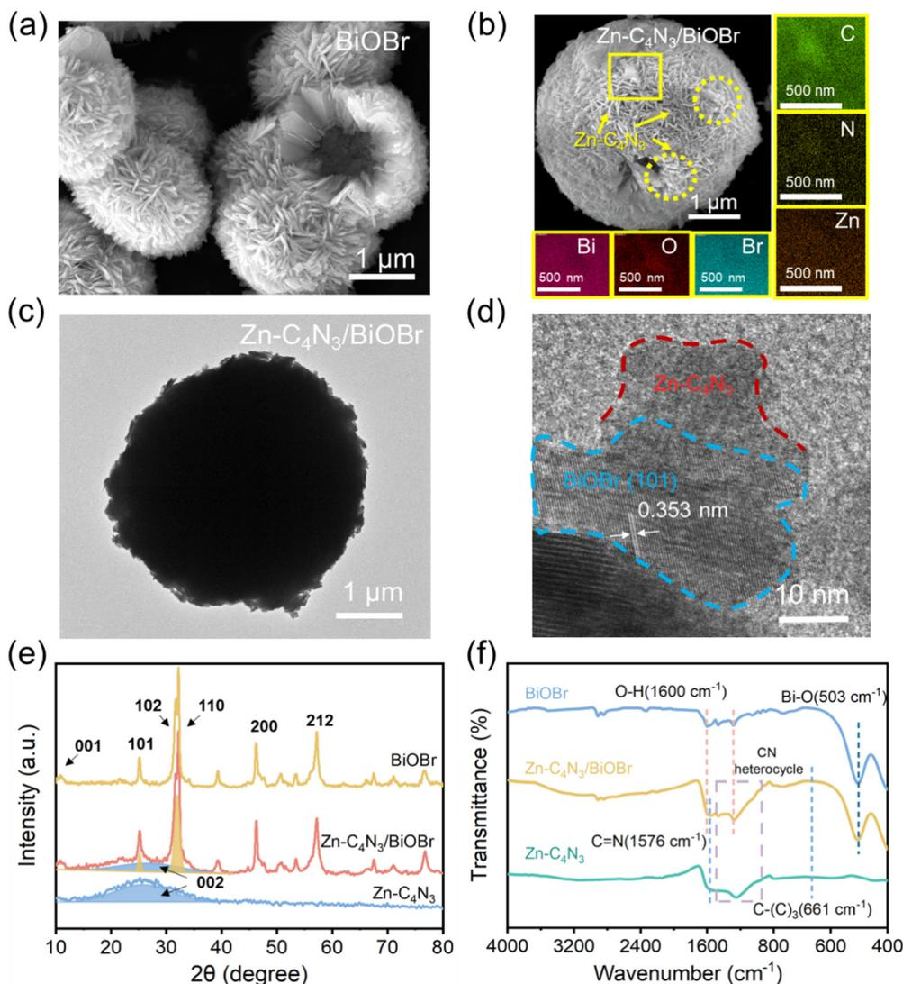
Fig. 1 (a) SEM image of BiOBr and (b) SEM image and EDS elemental mapping images of Zn-C<sub>4</sub>N<sub>3</sub>/BiOBr. (c) The whole TEM image of Zn-C<sub>4</sub>N<sub>3</sub>/BiOBr. (d) HRTEM images of the selected areas of Zn-C<sub>4</sub>N<sub>3</sub>/BiOBr. (e) XRD patterns and (f) FTIR spectra of Zn-C<sub>4</sub>N<sub>3</sub>, BiOBr and Zn-C<sub>4</sub>N<sub>3</sub>/BiOBr.
