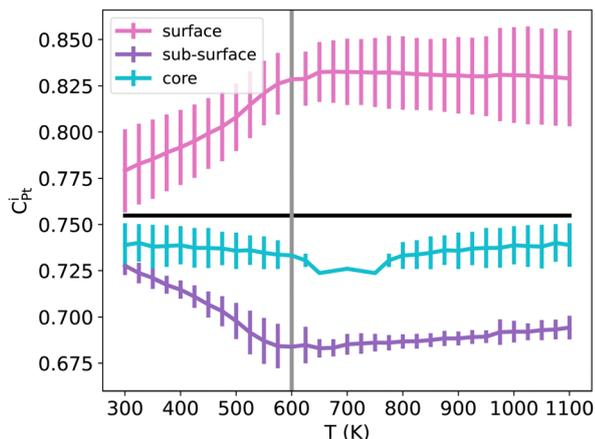
Fig. 13 NiPt<sub>3</sub> surface, sub-surface and core Pt concentration per atomic site as a function of temperature in the TOh<sub>1289</sub> nanoparticle. The horizontal black line represents the average Pt concentration while vertical the grey line represents the order/disorder transition temperatures. Error bars have a width of two standard deviations, calculated over a total of 40 independent runs. The solid line is obtained by averaging over the different runs.
