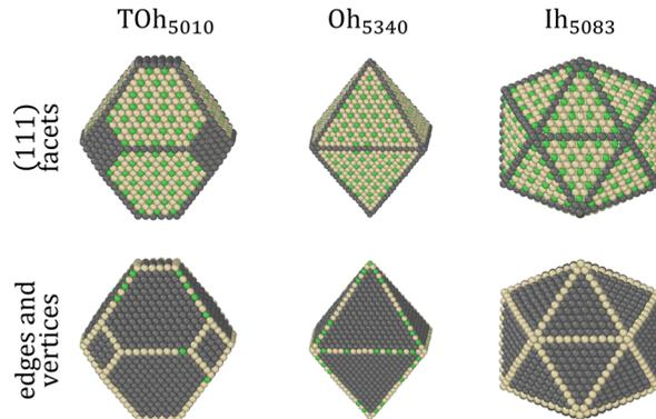
Fig. 11 Equilibrium chemical ordering states at 300 K in  $NiPt_3$  NPs on the  $\{111\}$  facets (top) and on the edges and vertices (bottom), for different NP shapes of similar size ( $TOh_{5010}$ ,  $Oh_{5340}$  and  $Ih_{5083}$ ). Ni atoms are colored in green, and Pt in beige. For all NP shapes, a  $p(2 \times 2)$   $\{111\}$  surface ordering compatible with the  $L1_2$  core ordering is observed.
