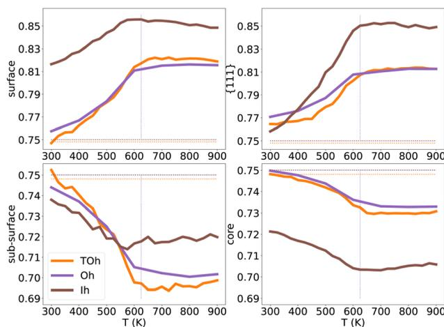
Fig. 12  $NiPt_3$  surface,  $\{111\}$  facets, subsurface and core Pt concentration per site as a function of temperature for the three NP shapes  $TOh_{5010}$  (orange),  $Oh_{5340}$  (purple) and  $Ih_{5083}$  (brown), shown in Fig. 11. Horizontal lines represent the average Pt concentration. Vertical lines represent the critical transition temperature, which here is the same regardless of shapes.
