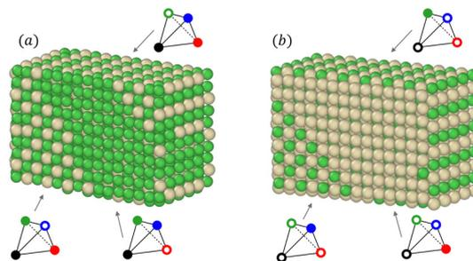
**Fig. 7** Snapshots of slices from the core of (a) Ni<sub>3</sub>Pt and (b) NiPt<sub>3</sub> TOh<sub>5010</sub> nanoparticles at 300 K. Same labels (a) and (b) are reported in Fig. 6 for clarity. The three arrows point towards three different L<sub>12</sub> translation variants which coexist in the cores of the NPs for this rather large NP size. The associated chemical occupation is given in the tetrahedron schemes, following the same conventions as in Fig. 6.
