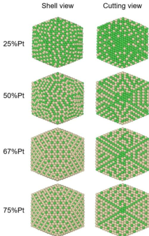
Fig. 10 Snapshots of  $Ih_{5083}$  NPs at different compositions and after thermal equilibration at 300 K, showing the chemical ordering from a shell view (left column) and a cutting view (right column). Green atoms represent Ni and beige atoms represent Pt.
