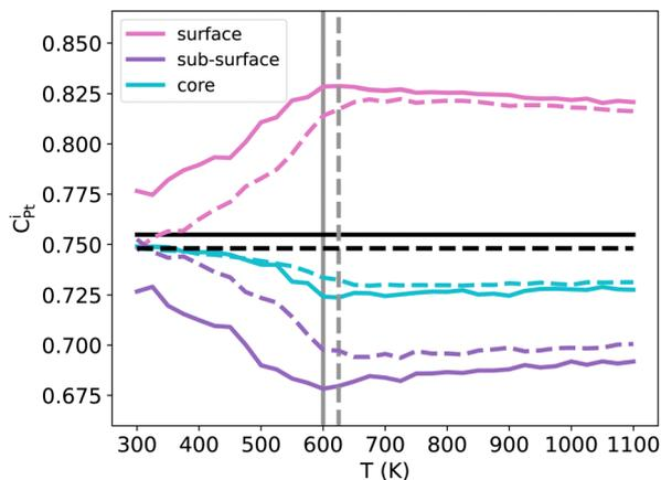
Fig. 9 NiPt<sub>3</sub> surface, sub-surface and core Pt concentration per atomic site as a function of temperature in TOh<sub>1289</sub> (solid lines) and TOh<sub>5010</sub> (dashed lines) nanoparticles. Horizontal black lines represent the average Pt concentration while vertical grey lines represent the order/disorder transition temperatures of both NP sizes.
