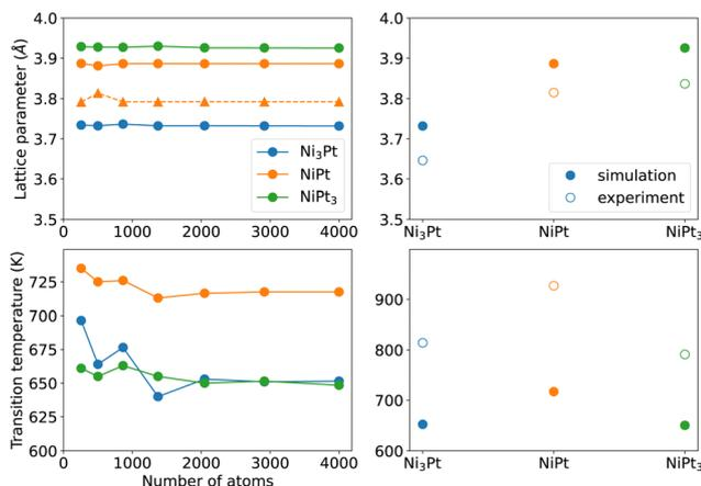
Fig. 2 Bulk lattice parameters at 300 K (top left with circles for  $a$  and triangles for  $c$  lattice constants) and critical order/disorder transition temperatures (bottom left) of the  $\text{Ni}_3\text{Pt}$ ,  $\text{NiPt}$  and  $\text{NiPt}_3$  ordered alloys, as a function of the number of atoms in the simulation box. The right panels compare their converged values to the experimental ones.<sup>40–43</sup>
