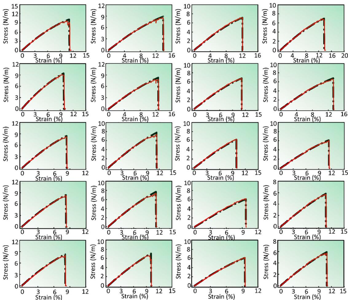
Fig. 7 XGBoost model prediction to capture the variation for different chalcogens O, S, Se, and Te (left to right) along with varying defects pristine,  $V_{2C}$ ,  $V_C$ ,  $V_M$ , and  $V_{M-2C}$  (top to bottom). The transition metal and strain rate are fixed as vanadium (V) and  $10^8 \text{ s}^{-1}$ , respectively. All the subfigures present stress–strain responses in the armchair direction.
