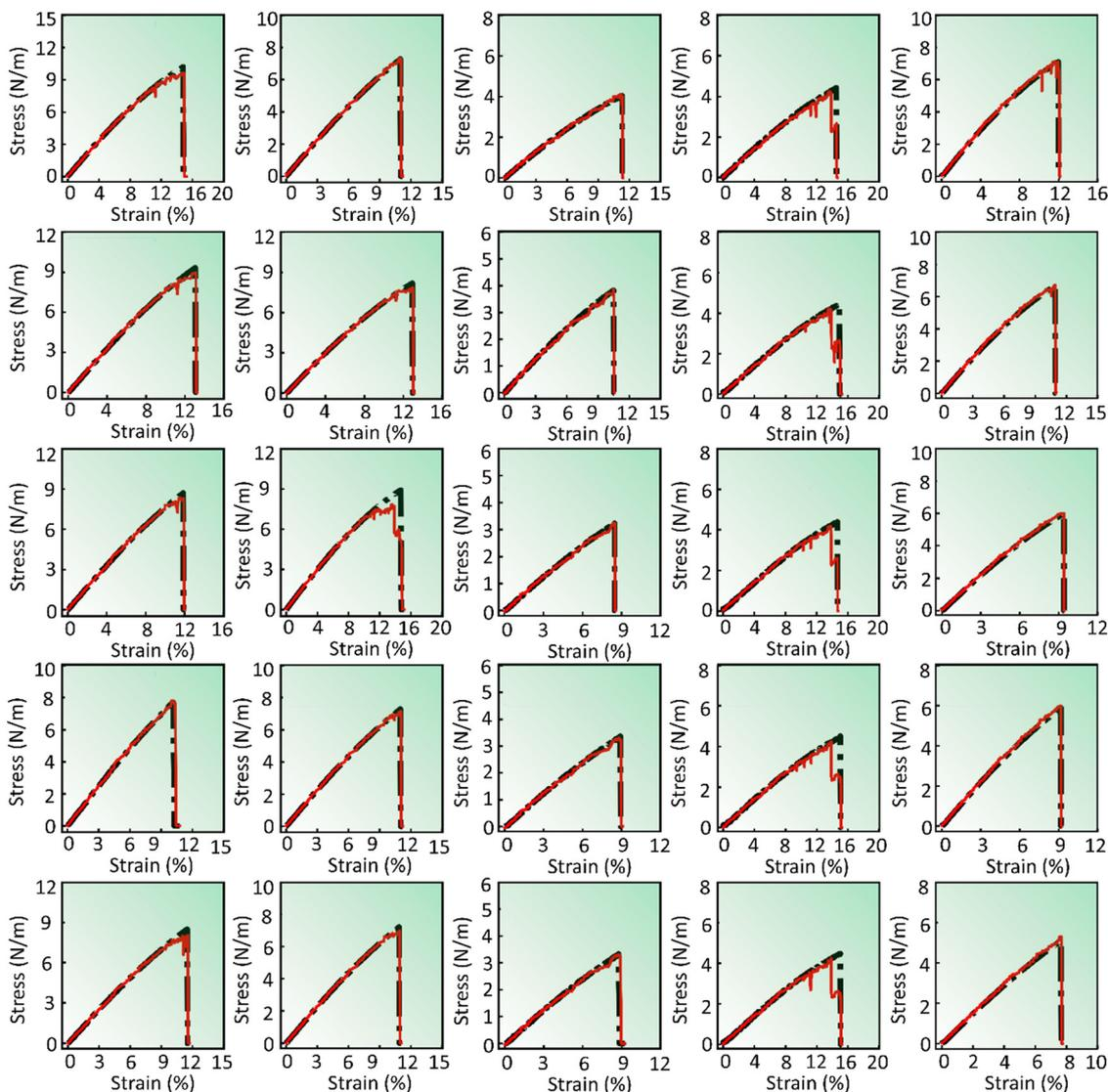
Fig. 8 XGBoost model prediction to capture the variation for different metals Cr, Nb, Ni, Sc, and V (left to right) along with varying defects pristine,  $V_{2C}$ ,  $V_C$ ,  $V_M$ , and  $V_{M-2C}$  (top to bottom). The chalcogen and strain rate are fixed as Se and  $10^7 \text{ s}^{-1}$ , respectively. All the subfigures present stress–strain responses in the armchair direction.
