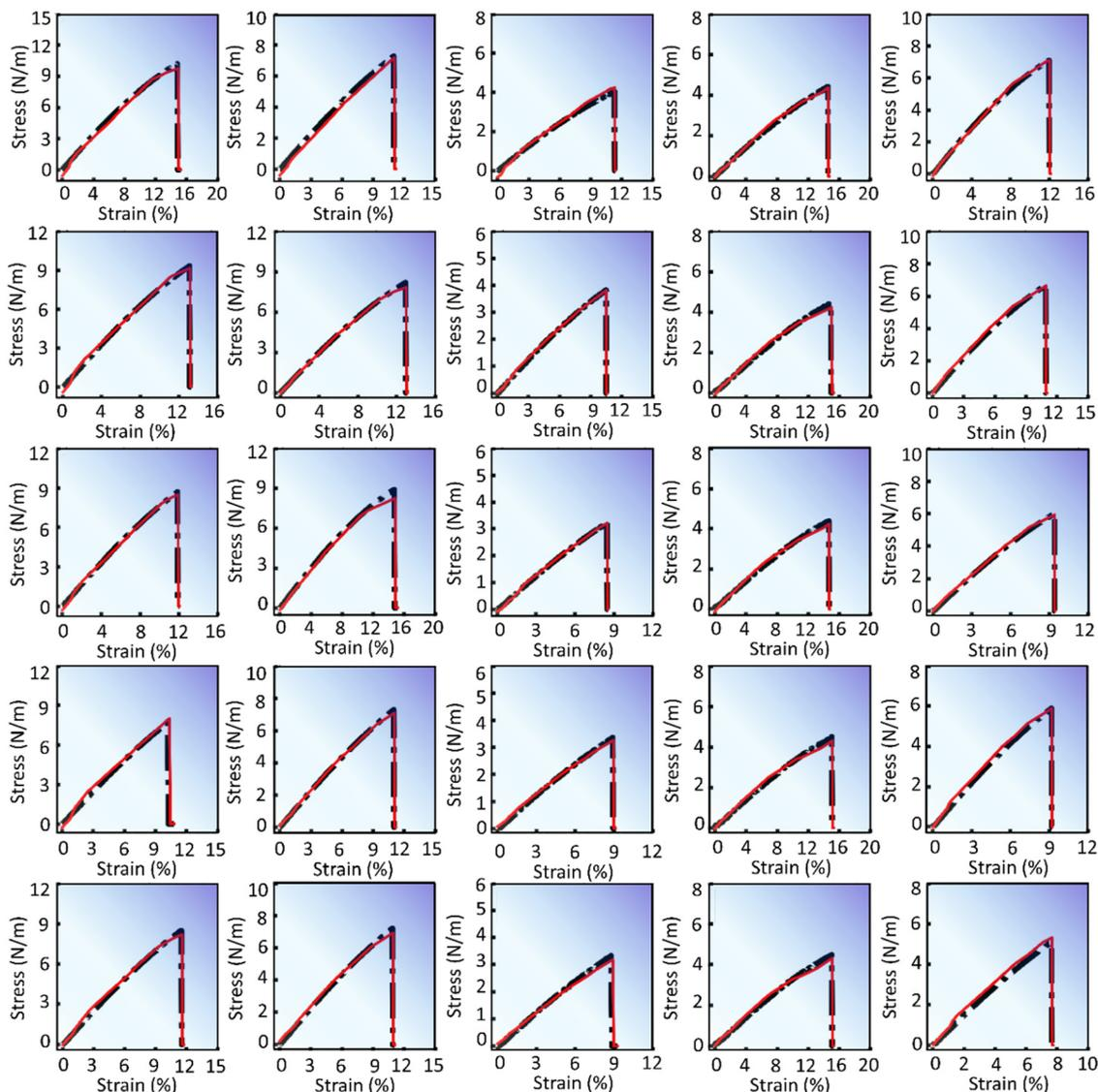
Fig. 5 DenseNet model predictions to capture the variation for different metals Cr, Nb, Ni, Sc, and V (left to right) along with varying defects pristine,  $V_{2C}$ ,  $V_C$ ,  $V_M$ , and  $V_{1M-2C}$  (top to bottom). The chalcogen and strain rate are fixed as Se and  $10^7 \text{ s}^{-1}$ , respectively. All the subfigures present stress–strain responses in the armchair direction.
