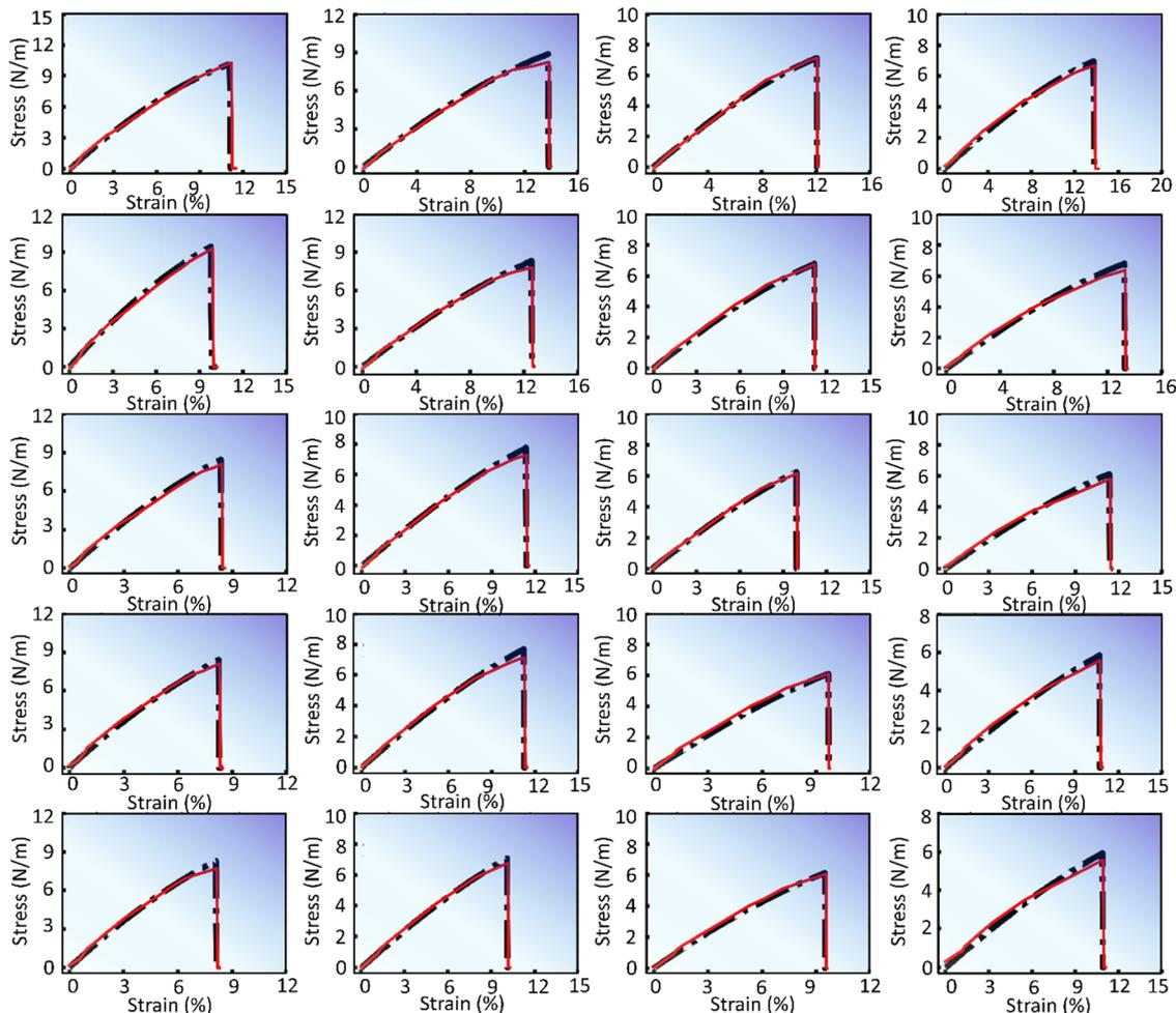
Fig. 4 DenseNet model predictions to capture the variation for different chalcogens O, S, Se, and Te (left to right) along with varying defects pristine,  $V_{2C}$ ,  $V_C$ ,  $V_M$ , and  $V_{1M-2C}$  (top to bottom). The transition metal and strain rate are fixed as vanadium (V) and  $10^8 \text{ s}^{-1}$ , respectively. All the subfigures present stress–strain responses in the armchair direction.
