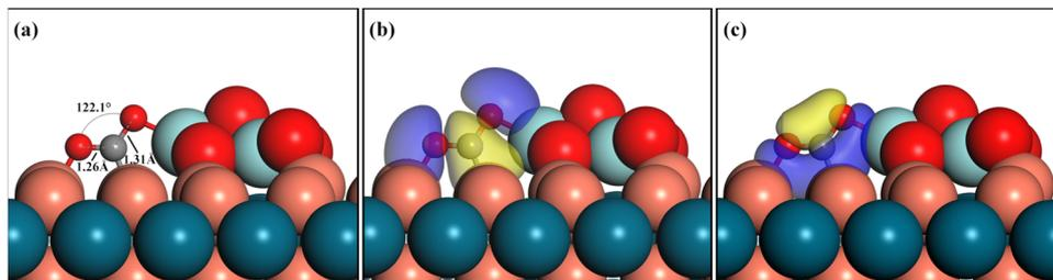
Fig. 3 (a) Geometry configuration and (b) and (c) calculated isosurfaces of the bonding orbital for CO<sub>2</sub> adsorbed on Z/CuPd(100)-Cu, where blue represents the negative lobe, while yellow represents the positive lobe. Cu: orange, Pd: dark blue, Zr: light blue, O: red and C: grey.
