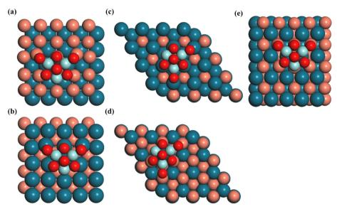
Fig. 1 Top views of the DFT-optimized structures of the inverse catalysts for (a) Zr<sub>3</sub>O<sub>6</sub>/CuPd(100)-Cu, (b) Zr<sub>3</sub>O<sub>6</sub>/CuPd(100)-Pd, (c) Zr<sub>3</sub>O<sub>6</sub>/CuPd(111)-Pd, (d)  $Zr_3O_6/CuPd(111)$  – Cu, (e)  $Zr_3O_6/CuPd(110)$ . Cu: orange, Pd: dark blue, Zr: light blue and O: red.
