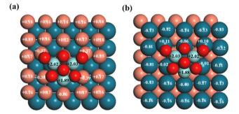
Fig. 2 Bader charge analysis (in |e|) of (a) Z/CuPd(100)–Cu and (b) Z/CuPd(100)–Pd. The numbers on the atoms are the calculated charge transfer from the Bader charge analysis.
