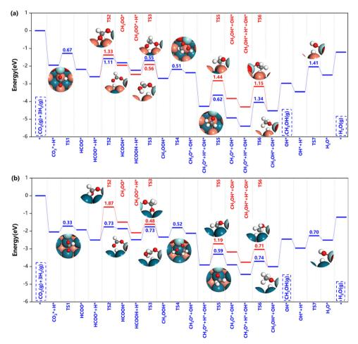
Fig. 6 Potential energy diagrams and corresponding transition state structures of methanol formation over (a) Z/CuPd(100) - Cu and (b) Z/CuPd(100) -Pd on the formate pathway
