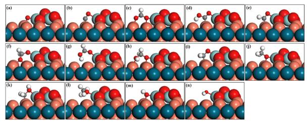
Fig. 4 Adsorbed structures of the intermediates involved in the synthesis of methanol through CO<sub>2</sub> hydrogenation over Z/CuPd(100)-Cu. (a) O\*. (b) CO\*, (c) HCOO\*, (d) COOH\*, (e) HCO\*, (f) CH<sub>2</sub>OO\*, (g) HCOOH\*, (h) CH<sub>2</sub>OOH\*, (i) CH<sub>2</sub>O\*, (j) CH<sub>3</sub>O\*, (k) CH<sub>2</sub>OH\*, (l) OH\*, (m) OH\*, (m) OH\*, (n) H<sub>2</sub>O\*. Cu: orange, Pd: dark blue, Zr: light blue, O: red and C: grey
