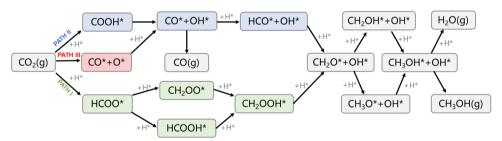
Fig. 5 Reaction network for CO<sub>2</sub> hydrogenation to methanol and carbon monoxide over Zr<sub>3</sub>O<sub>6</sub>/CuPd inverse catalysts. PATH I: formate, PATH II: RWGS + CO-hydro, PATH III: CO<sub>2</sub> direct activation.
