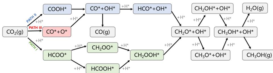
Fig. 5 Reaction network for CO<sub>2</sub> hydrogenation to methanol and carbon monoxide over Zr<sub>3</sub>O<sub>6</sub>/CuPd inverse catalysts. PATH I: formate, PATH II: RWGS + CO-hydro, PATH III: CO<sub>2</sub> direct activation.
