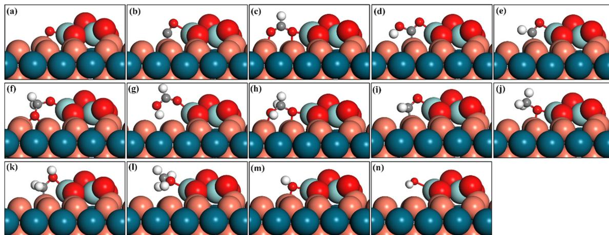
Fig. 4 Adsorbed structures of the intermediates involved in the synthesis of methanol through CO<sub>2</sub> hydrogenation over Z/CuPd(100)-Cu. (a) O\*, (b) CO\*, (c) HCOO\*, (d) COOH\*, (e) HCO\*, (f) CH<sub>2</sub>OO\*, (g) HCOOH\*, (h) CH<sub>2</sub>OOH\*, (i) CH<sub>2</sub>O\*, (j) CH<sub>3</sub>O\*, (k) CH<sub>2</sub>OH\*, (l) OH\*, (m) OH\*, (n) H<sub>2</sub>O\*. Cu: orange, Pd: dark blue, Zr: light blue, O: red and C: grey.
