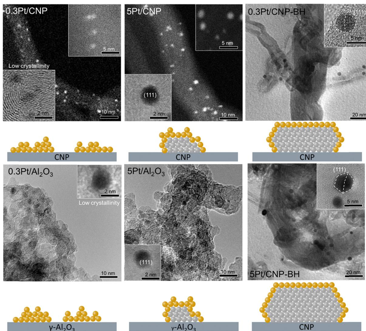
Fig. 10 HAADF STEM and HRTEM for the catalysts supported on CNP and Al<sub>2</sub>O<sub>3</sub>. Illustration of the structure of Pt nanoparticles: yellow and grey spheres represent the surface and bulk Pt atoms, respectively.
