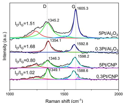
Fig. 9 Raman spectra of the catalysts after *n*-butane dehydrogenation reaction.
