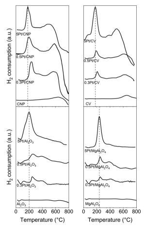
Fig. 4 TPR profiles of the samples.
