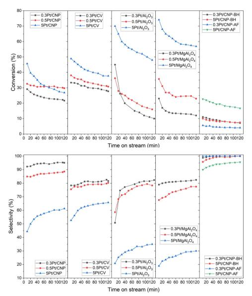
Fig. 7 Conversion and selectivity for all catalysts for *n*-butane dehydrogenation.
