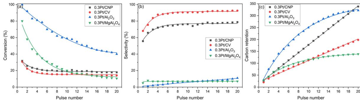
Fig. 8 *n*-Butane dehydrogenation reaction results as a function of the number of pulses.
