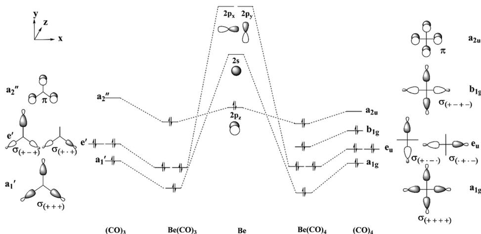
**Scheme 2** Atomic orbitals of Be atom in the excited state (1s<sup>2</sup>2s<sup>0</sup>2p<sub>z</sub><sup>2</sup>) interacting with ligands group orbitals of (CO)<sub>3</sub> and (CO)<sub>4</sub> fragments in Be(CO)<sub>3</sub> and Be(CO)<sub>4</sub>.
