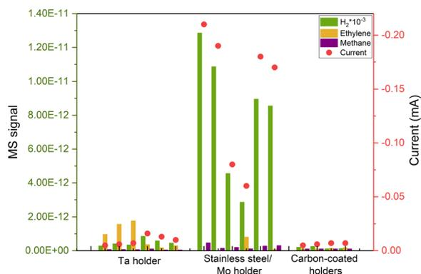
Fig. 5 Repetitions of COR of the same deposited sample (5 nm 5% coverage Cu nanoparticles), with different responses due to induced contamination from the UHV cleaning method. The results became reproducible after covering the electrode's holder with carbon. All measurements are done at the same applied potential of  $-0.75 V_{RHE}$ .
