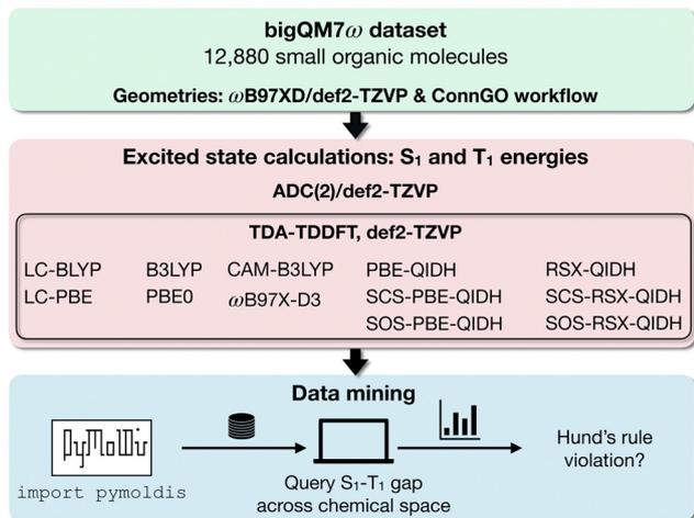
Fig. 1 Workflow outlining the design of the pymoldis module<sup>26</sup> for data mining  $S_1$  and  $T_1$  energies across 12 880 molecules with up to 7 CONF atoms in the bigQM7 $\omega$  dataset.<sup>27</sup> ADC(2) and TDDFT calculations were performed as a part of the present work. See (ESI<sup>†</sup>) for screenshots of example queries.
