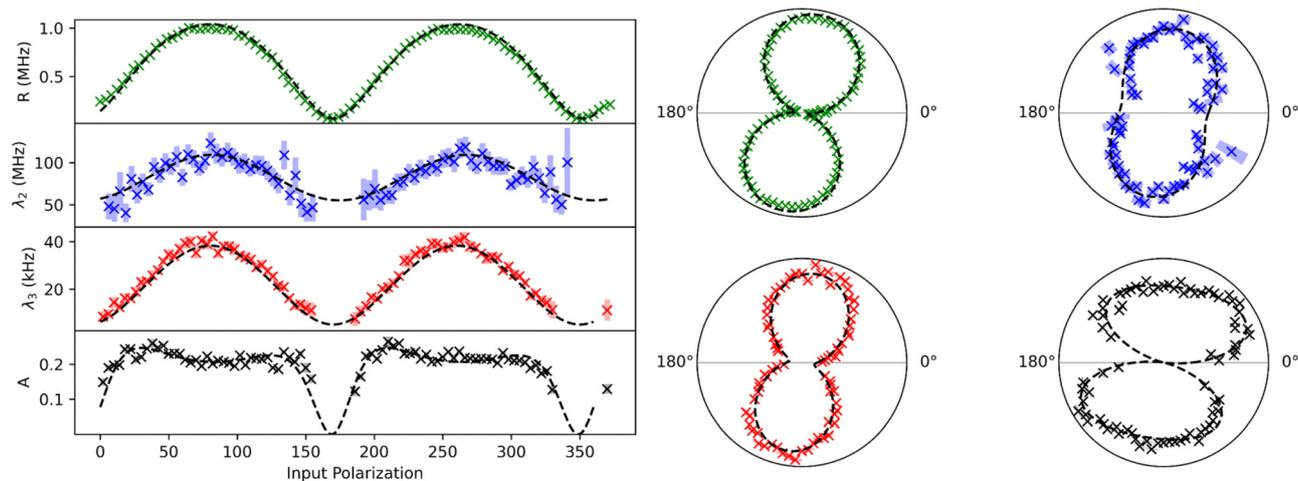
Fig. 3 Evolution of  $R$ ,  $\lambda_2$ ,  $\lambda_3$  and  $A$  as a function of input polarization angle for an in-phase (ip) molecule. Colored markers are experimental data points. Dashed black lines are result of a global fit function (see text for details). The colored areas represent the 68% confidence intervals of the second order correlation function fit results. Left and right panels are respectively linear and polar representation of the same data.
