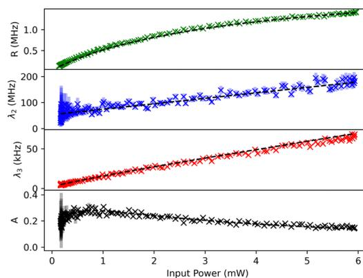
Fig. 2 Typical evolution of the measured count rates  $R$ ,  $\lambda_2$ ,  $\lambda_3$  and the bunching amplitude A as a function of excitation power (ramping up and down). The colored areas represent the 68% confidence intervals of the second order correlation function fit results. Dashed black lines are result of a global fit function (see text for details).
