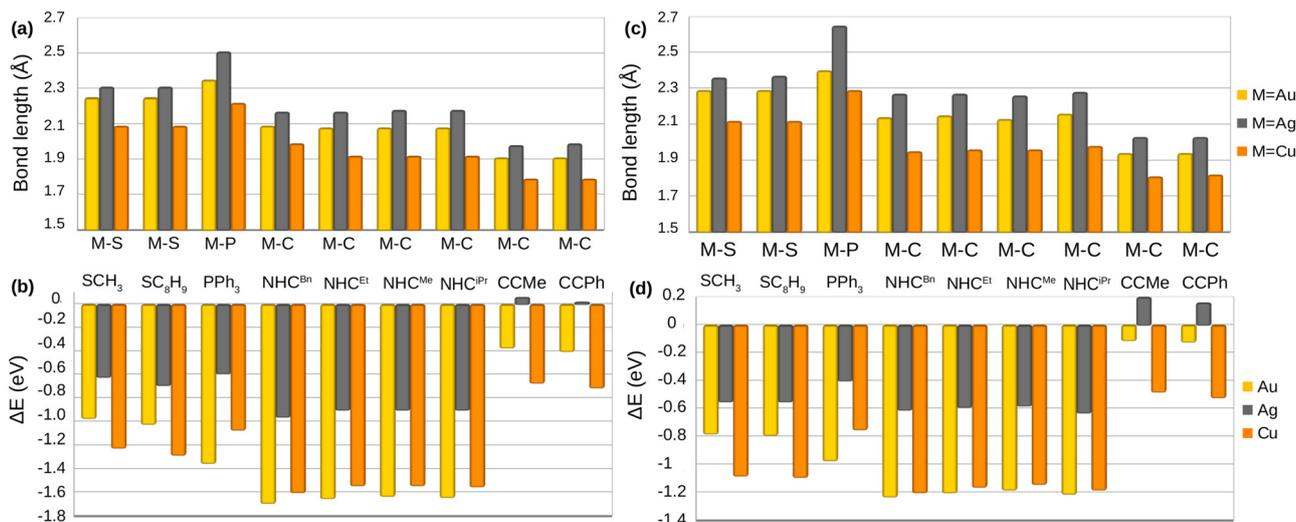
Fig. 2 Bond length M–L (Å) and binding energy (eV) calculated by PBE (shown in (a) and (b)) and BEEF-vdW (shown in (c) and (d)) for the M–L complexes. Table S2 (ESI<sup>†</sup>) contains the numeric values.
