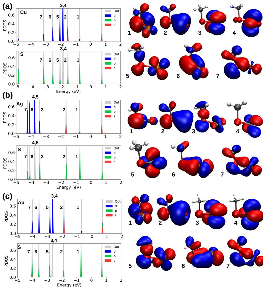
Fig. 3 Projected density of states along with the occupied molecular orbitals (the numbers 1 to 7 for refer to HOMO to HOMO–6) for (a) Cu–SCH<sub>3</sub> (b) Ag–SCH<sub>3</sub> and (c) Au–SCH<sub>3</sub>. The HOMO–LUMO gaps (centered around zero) are 1.48, 1.49, and 1.41 eV for systems a through c, respectively.
