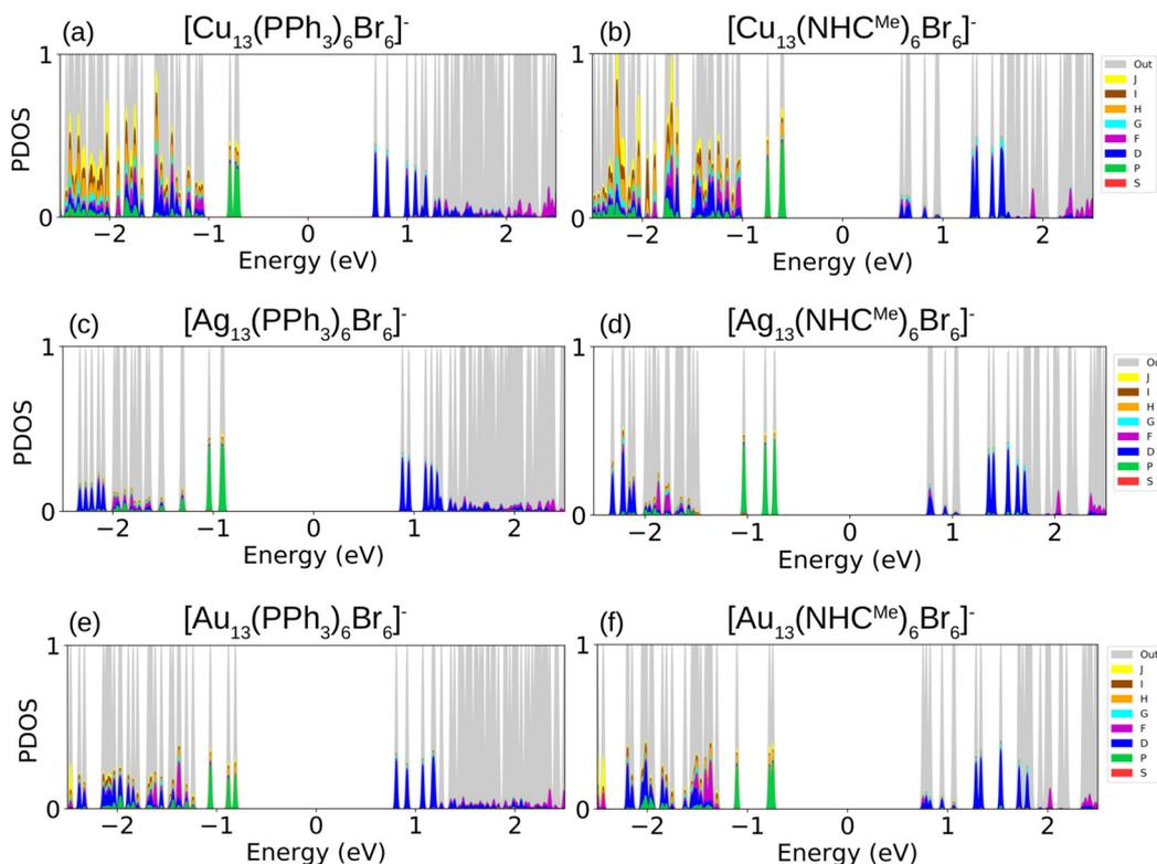
**Fig. 5** Projected density of states for (a)  $[Cu_{13}(PPh_3)_6Br_6]^-$ , (b)  $[Cu_{13}(NHC^{Me})_6Br_6]^-$ , (c)  $[Ag_{13}(PPh_3)_6Br_6]^-$ , (d)  $[Ag_{13}(NHC^{Me})_6Br_6]^-$ , (e)  $[Au_{13}(PPh_3)_6Br_6]^-$ , (f)  $[Au_{13}(NHC^{Me})_6Br_6]^-$ . The HOMO–LUMO gaps are 1.39, 1.18, 1.78, 1.51, 1.62, and 1.50 eV in a–f, respectively.
