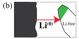
Fig. 6 (a) Schematic of a discharging lithium-ion battery. Li<sup>+</sup> ions and electrons flow from a lithium metal anode to a cathode particle converting from the delithiated to the lithiated phase (shaded white and green, respectively). (b) Simplified process, chemically and energetically equivalent to that in (a), with a transfer of lithium atoms from anode to cathode.
