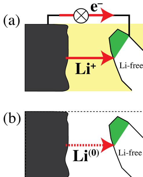
Fig. 6 (a) Schematic of a discharging lithium-ion battery.  $\text{Li}^+$  ions and electrons flow from a lithium metal anode to a cathode particle converting from the delithiated to the lithiated phase (shaded white and green, respectively). (b) Simplified process, chemically and energetically equivalent to that in (a), with a transfer of lithium atoms from anode to cathode.
