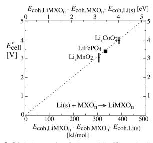
Fig. 3 Relation between the cell voltage and the difference in cohesive energies of a lithium-metal anode and the two phases in the cathode, for three types of cathodes. The theoretically expected relation (without a free factor) is indicated by the dashed line. Note that E stands for energy on the horizontal and for electromotive force on the vertical axis. For cohesive energies see Section 4 of the ESI,† while the cell voltage data were taken from ref. 2 and 10
