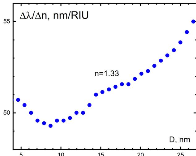
Fig. 23 Dependence of the refractive index sensitivity (RIS) of Au nanoparticles with sizes 5–27 nm at the refractive index of aqueous medium ( $n = 1.33$ ). The Mie theory calculations with size correction for the Au dielectric constants by Karimi.<sup>130</sup> From ref. 124.
