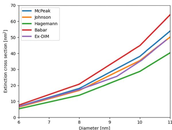
Fig. 2 The extinction cross section as a function of size for the Ex-DIM and Mie theory with different experimental inputs for the dielectric constant. The size correction in the Mie theory is taken from Karimi *et al.*<sup>130</sup> The different experimental input data are from bulk or thick films from McPeak *et al.*,<sup>133</sup> Johnson and Christy,<sup>134</sup> Hagemann *et al.*<sup>132</sup> and Babar *et al.*<sup>131</sup>
