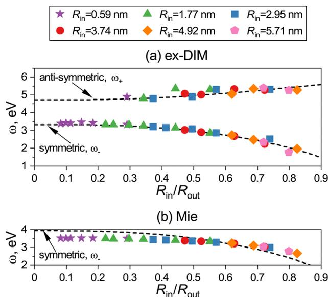
Fig. 10 The spectral positions of SPRs for the symmetric and anti-symmetric modes versus  $R_{in}/R_{out}$  calculated via (a) Ex-DIM and (b) Mie theory for nano-shells with different  $R_{in}$ . The dashed line shows the spectral position of symmetric,  $\omega_-$ , and anti-symmetric,  $\omega_+$ , modes from eqn (1) in ref. 143 with (a)  $\omega_B = 5.78$  eV and (b) 6.82 eV used for the fit. From ref. 143.
