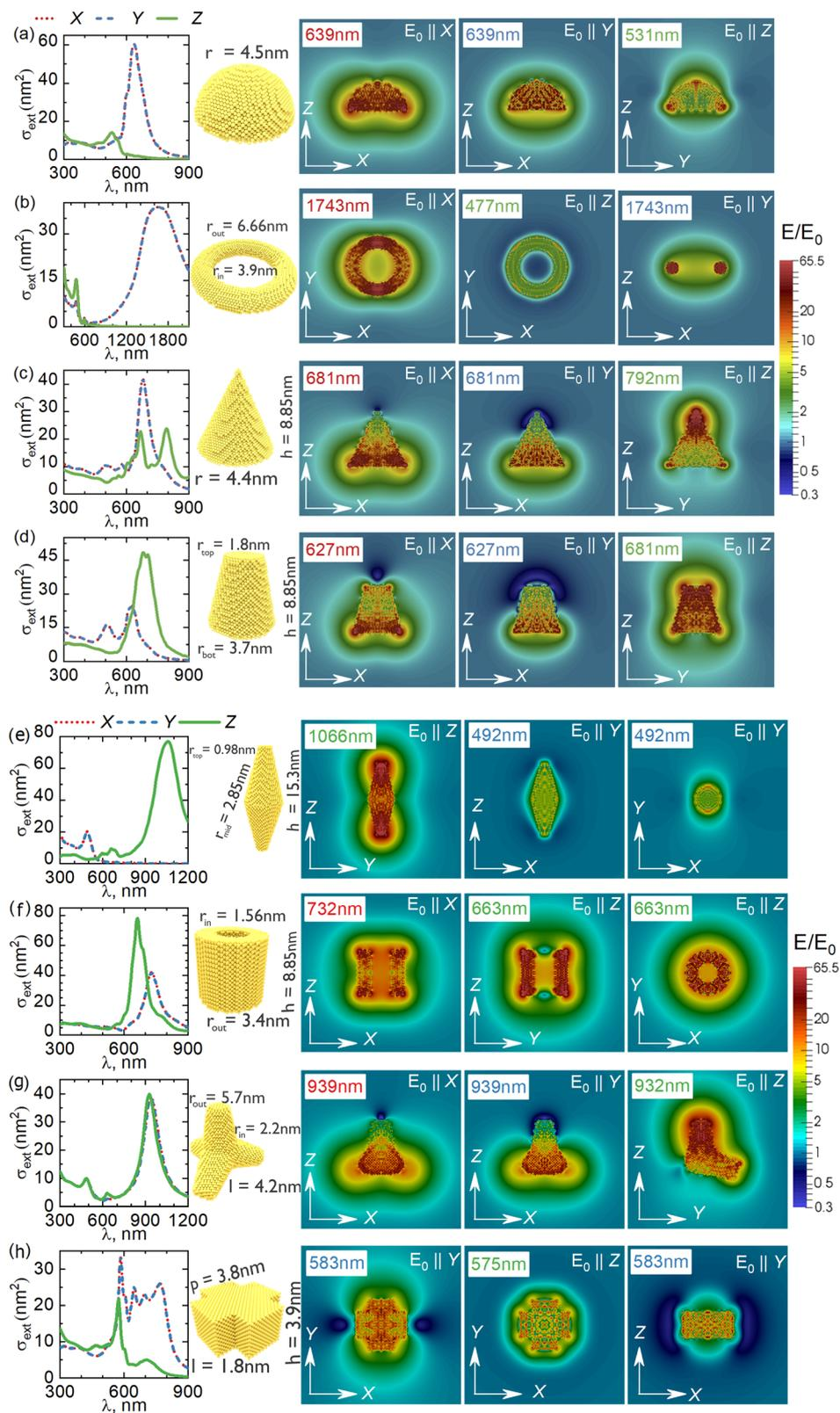
Fig. 16 Plasmonic electric fields from polarized external electric fields together with spectra for ultra-fine plasmonic nanoparticles of different shape. From ref. 152.
