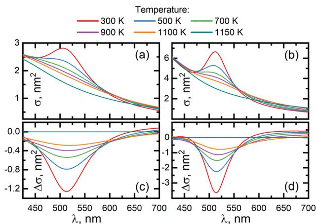
**Fig. 29** Extinction spectra variation for the 6 nm Au nanoparticle with suppression of surface plasmon resonance in the temperature range 300–1150 K (Ex-DIM calculations). Variation of differential extinction spectra with suppression of surface plasmon resonance in for temperatures 300–1150 K (all curves were subtracted from the spectral dependence for  $T = 1150$  K). (a) and (b) In vacuum, (b) and (d) in medium with refractive index  $n_0 = 1.33$  (b). From ref. 196.
