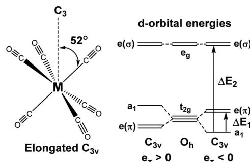
Fig. 6 Trigonal distortion applied to M(CO)<sub>6</sub> compounds and relationship between the sense of splitting of the t<sub>2g</sub> orbitals and the sign of the  $e_{\pi}$  parameter.
