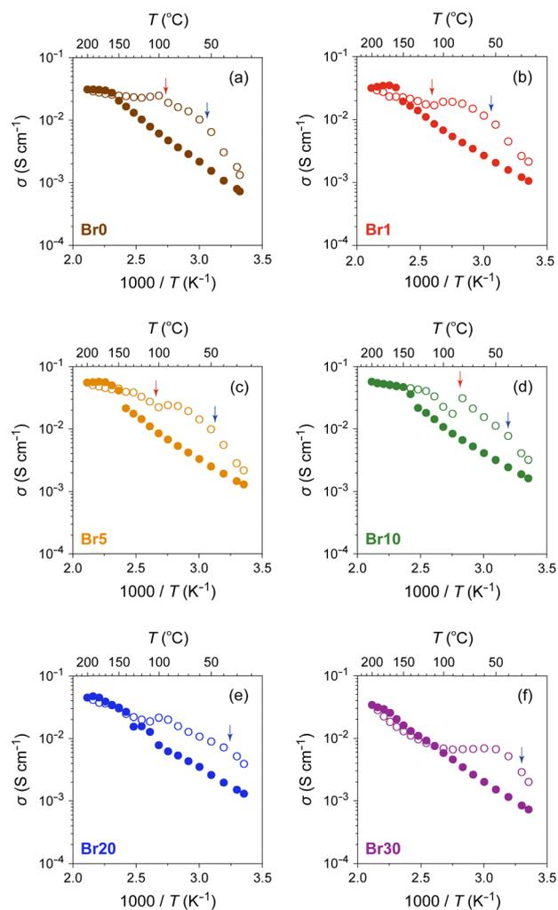
**Fig. 6** Temperature dependence of  $\sigma$  for  $\text{AgI}$ - $\text{AgBr}$ /MPA composites with various  $\text{AgI}:\text{AgBr}$  molar ratios ((a) **Br0**, (b) **Br1**, (c) **Br5**, (d) **Br10**, (e) **Br20**, and (f) **Br30**) in heating (closed circles) and cooling (open circles) processes. The red and blue arrows indicate the onset temperatures of the transition on the high- and low-temperature sides, respectively, in the DSC cooling process (Fig. 3).
