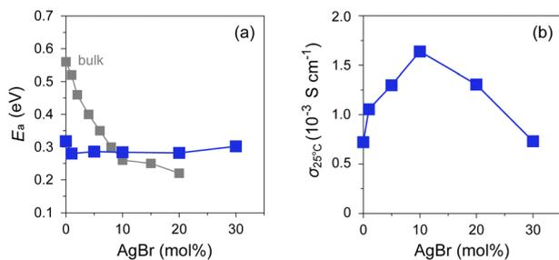
Fig. 7 Plots of (a)  $E_a$  and (b)  $\sigma_{25^\circ\text{C}}$  against AgBr-doping ratio for AgI–AgBr/MPA composites represented by closed blue squares. Closed grey squares represent the values of bulk AgI–AgBr mixed crystals.<sup>49–51,78</sup>
