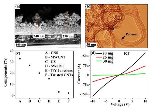
Fig. 6 (a) Cross-sectional SEM image of a coated film with 30 mg polyurethane binder. The thickness of the film is  $250 \pm 10 \mu m$ . (b) TEM image of polymer-grafted CNTs revealing a polymer thickness of around 10-20 nm. (c) Statistical weight percentage of different structural components present in the sample. (d) Typical I-V characteristics exhibiting different conducting channels depending on the polymer content.
