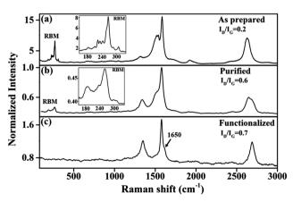
Fig. 3 Raman spectra of (a) as-prepared, (b) purified and (c) functionalized samples. The spectra are normalized with respect to the G peak of the purified samples shown in (b). Insets of (a) and (b) reveal the RBM in the as-prepared and purified samples.
