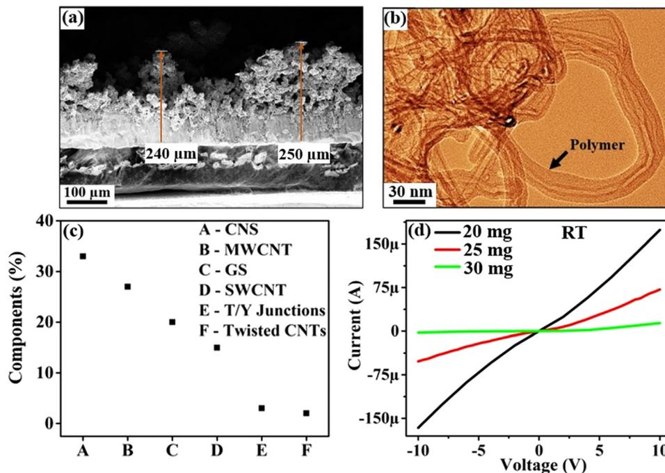
Fig. 6 (a) Cross-sectional SEM image of a coated film with 30 mg polyurethane binder. The thickness of the film is  $250 \pm 10 \mu\text{m}$ . (b) TEM image of polymer-grafted CNTs revealing a polymer thickness of around 10–20 nm. (c) Statistical weight percentage of different structural components present in the sample. (d) Typical  $I$ - $V$  characteristics exhibiting different conducting channels depending on the polymer content.
