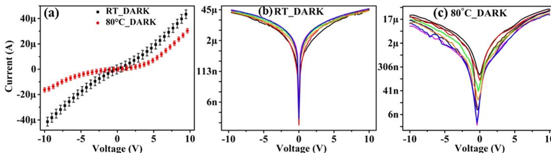
Fig. 7 Two-probe electrical measurements at RT and  $80^\circ\text{C}$  on the coated film in the dark. (a) Overall  $I$ - $V$  characteristics. Each spectrum is an average of 10 data sets. (b) and (c) Natural log of current vs. voltage plots. There are many data sets (8–10) in each graph shown in different colours, validating the repeatability of the measurement.
