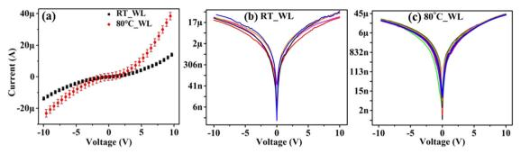
Fig. 8 Two-probe electrical measurements at RT and 80 °C under WL exposure. (a) Overall I-V characteristics. Each curve corresponds to an average of 20 data sets. The experimental error lies within the limit. Natural log of current vs. voltage plots. There are 6 data sets in (b) and 26 data sets in (c) denoted in different colours to show the consistent electrical behaviour of the sample.
