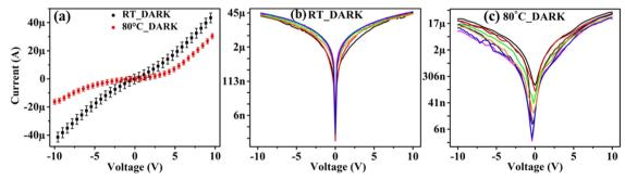
Fig. 7 Two-probe electrical measurements at RT and 80 °C on the coated film in the dark. (a) Overall I-V characteristics. Each spectrum is an average of 10 data sets. (b) and (c) Natural log of current vs. voltage plots. There are many data sets (8-10) in each graph shown in different colours, validating the repeatability of the measurement.
