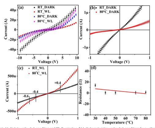
Fig. 9 (a) Consolidated I-V plots under dark condition and WL illumination. (b) I-V characteristics under dark conditions for a voltage range of  $\pm 1$  V. (c) I-V data under WL exposure for a voltage range of ±1 V. A rise in the current after certain voltages is denoted in the plot. (d) Resistance vs. temperature plot displaying the semiconducting nature of the film
