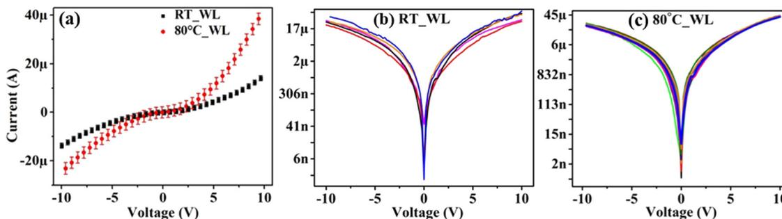
Fig. 8 Two-probe electrical measurements at RT and 80 °C under WL exposure. (a) Overall  $I$ - $V$  characteristics. Each curve corresponds to an average of 20 data sets. The experimental error lies within the limit. Natural log of current vs. voltage plots. There are 6 data sets in (b) and 26 data sets in (c) denoted in different colours to show the consistent electrical behaviour of the sample.
