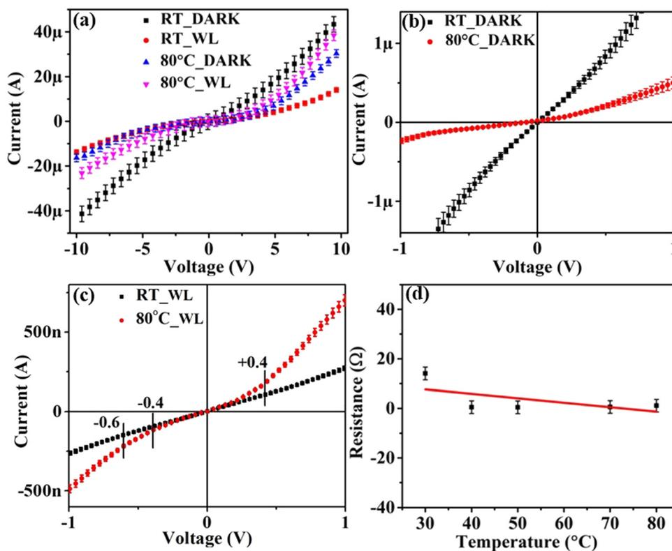
Fig. 9 (a) Consolidated  $I$ - $V$  plots under dark condition and WL illumination. (b)  $I$ - $V$  characteristics under dark conditions for a voltage range of  $\pm 1$  V. (c)  $I$ - $V$  data under WL exposure for a voltage range of  $\pm 1$  V. A rise in the current after certain voltages is denoted in the plot. (d) Resistance vs. temperature plot displaying the semiconducting nature of the film.
