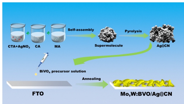
Scheme 1 Schematic illustration of the fabrication process of Mo,W:BVO/Ag@CN.
