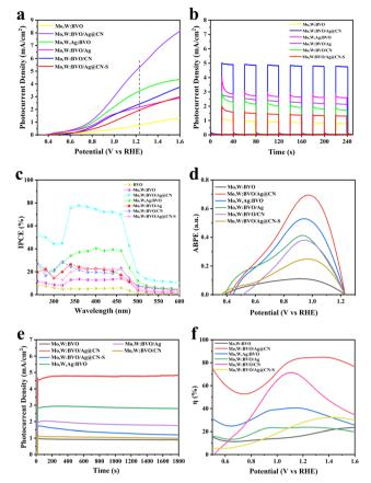
Fig. 3 (a) LSV examination, (b) I-T curves, (c) IPCE curves and (d) ABPE curves, (e) stability curves, (f) charge transfer efficiency of BVObased samples.
