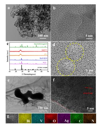
Fig. 1 Ag@CN of (a) TEM image and (b) HRTEM image; (c) XRD patterns of Mo,W:BVO/Ag@CN, BVO, Mo,W:BVO, CN and Ag@CN; Mo,W:BVO/ Ag@CN of (d) SEM image, (e) TEM image, (f) HRTEM image, (g) EDS elemental mapping
