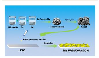
Scheme 1 Schematic illustration of the fabrication process Mo,W:BVO/Ag@CN.
