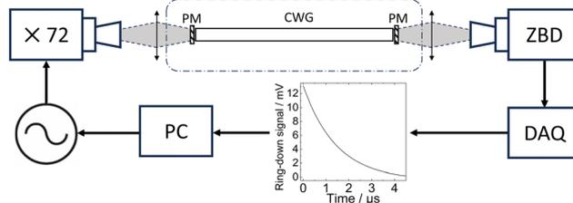
Fig. 1 THz cavity ring-down spectroscopy setup. An AMC source coupled to a resonant cavity itself composed of two photonic mirrors (PM) and a corrugated waveguide (CWG). The output of the cavity is measured by a ZBD whose signal is recorded using a data acquisition system (DAQ). The cavity is placed inside a low pressure gas chamber, as indicated by the dashed-dotted line.
