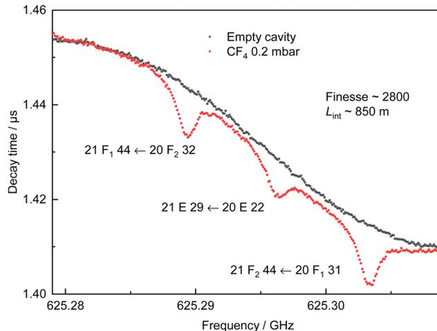
Fig. 2 A CRDS spectrum and its baseline probing 3 rotational transitions of  $\text{CF}_4$ . Black points, cavity under vacuum conditions. Red points,  $\text{CF}_4$  at 0.2 mbar. Each point is the average of  $10^5$  ring-down events. Step size 100 kHz, total acquisition time 600 s.
