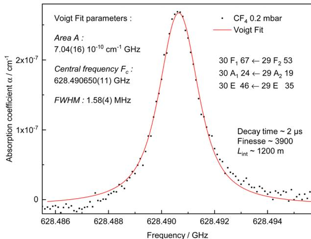
Fig. 4 Absorption spectrum of 3  $\text{CF}_4$  transitions, the line centred frequencies are separated by less than 100 kHz so they cannot be resolved due to the Doppler broadening. Acquisition with a step size of 100 kHz, and  $1 \times 10^5$  ring-down events are averaged to obtain a single frequency point, and a total acquisition time of 220 s is required to obtain a complete spectrum. A single Voigt function with a fixed Gaussian contribution is used to fit the absorption profile.
