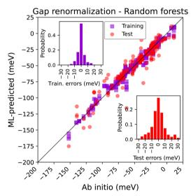
Fig. 3 Scatter plots: predictions of the renormalizations using random forests on top of linear regression vs. ab initio results. Histograms: training and test errors. Top: HOMO; center: LUMO; bottom: gap
