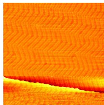
**Fig. 3** 150 nm  $\times$  150 nm STM image of the as-prepared Au(111) surface after 1 h in 0.8 bar argon, containing roughly 1 mbar of water, at room temperature. The image is taken in UHV at room temperature with  $-1$  V and 50 pA.
