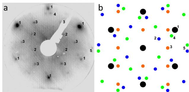
**Fig. 2** (a) LEED image taken of Au(111) after  $O_2$  exposure (78 eV electron energy). (b) Simulated LEED image based on the unit cell measured in STM including the Au(111) substrate in black and the three different possible orientations of the oxide overlayer in blue, orange, and green. Corresponding spots in (a) and (b) are marked with numbers 1 to 5. The simulated LEED image is made using LEEDpat.<sup>58</sup>
