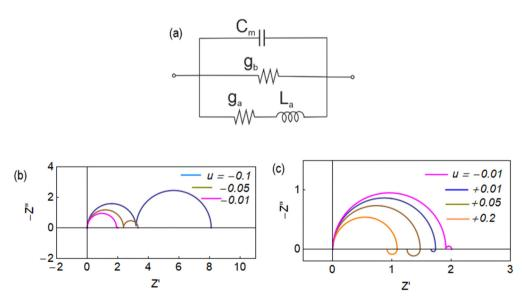
(a) Equivalent circuits and (b) and (c) impedance spectra at different stationary voltages. Same parameters as in Fig. 4 and  $C_{\rm m}=0.001$ .
