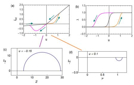
Fig. 5 Hysteresis at a rate  $v_{scan} = 10$  in (a) current-voltage curves and (b) state variable. The grey lines are the equilibrium curves. (c) and (d) Impedance spectra at the indicated voltage points. Parameters as in Fig. 4.
