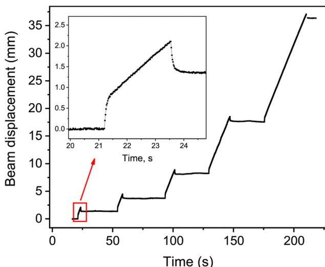
Fig. 2 Displacement of the reflected laser beam as a result of five exposure periods of different durations. Light source: 1 W LED 465 nm; crystal length 13 mm; and cross-section  $280 \times 350 \mu\text{m}$ . In the inset – enlarged image of the first exposure period.
