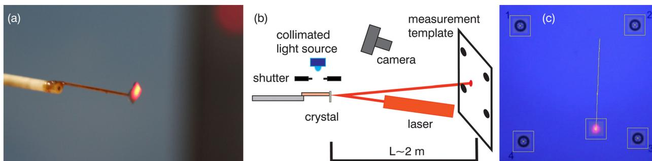
Fig. 1 Experimental setup: a cantilevered crystal (length 13 mm, cross-section  $280 \times 350$   $\mu\text{m}$ ) with a Si mirror at the free end (a), scheme of the experimental setup (b), and trajectory of the laser spot movement relative to the template marks (c).
