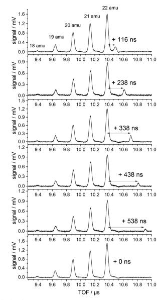
Fig. 3 TOF spectra in the region of the  $NH_{4-n}D_n$  cations produced with 226 nm excitation (lowest trace) and additional 266 nm excitation delayed by the indicated delay time.
