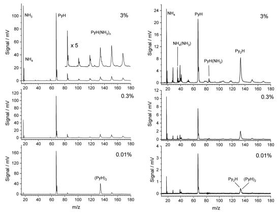
Fig. 1 Time-of-fight mass spectra of pyrrole in the presence of NH<sub>3</sub> ionized with 118 nm (left) and 226 nm (right) photons. The concentration of NH<sub>3</sub> in the carrier gas decreases from 3% (top) to 0.3% (middle) and less than 0.01% (bottom)
