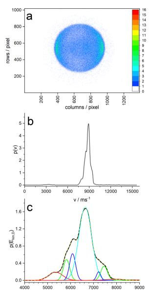
Fig. 5 (a) Ion image of the D-atoms produced by photodissociation of PyD with photons of 243 nm. (b) Velocity distribution of the D-atoms extracted from the ion image. (c) Kinetic energy distribution of the D-atoms and fit of 7 Gaussians.
