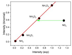
Fig. 4 Intensities predicted by a binomial distribution with p(D) = 0.7plotted against the experimental intensities of the  $NH_{4-n}D_n$  cation signals produced by 226 nm excitation. All intensities are normalized to the value for n = 3. The red line shows the expected behavior of the binomial distribution. The green arrow indicates the excess signal for ND<sub>4</sub>. The excess signal is 56% of the observed signal
