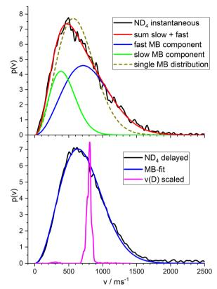
Fig. 6 (top) Velocity distribution obtained from ion images of ND<sub>4</sub> produced by two-photon absorption of 226 nm photons and fit with two MBDs. The fit with a single MBD is shown as dotted line. (bottom) Velocity distribution from consecutive absorption of one photon of 226 nm and a second photon of 266 nm, delayed by 300 ns and fit by a single MBD. The magenta curve is the expected velocity distribution for the impulsive model.
