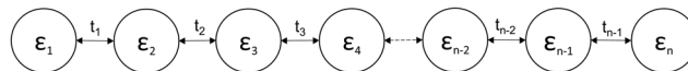
Fig. 2 A tight-binding model for conjugated molecule represented as an oligomer of length, n .
