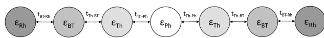
Fig. 12 Tight-binding model for IDTBR with tight-binding parameters – \epsilon_{\text{Ph}} , \epsilon_{\text{BT}} , \epsilon_{\text{Th}} and \epsilon_{\text{Rh}} , and hopping matrix elements – t_{\text{Th-Ph}} , t_{\text{Th-BT}} and t_{\text{BT-Rh}} .
