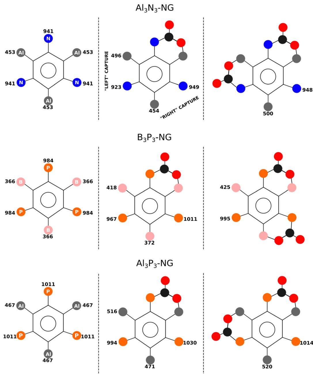
Fig. 6 FIA and PA of the different stationary points in kJ mol<sup>-1</sup>. The 2CO<sub>2</sub>-NG adduct associated with the lowest TS barrier is shown in the third column.
