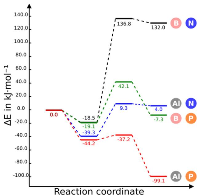
**Fig. 4** Energy profiles for the capture of one  $\text{CO}_2$  molecule by the  $\text{B}_3\text{N}_3\text{-NG}$ ,  $\text{B}_3\text{P}_3\text{-NG}$ ,  $\text{Al}_3\text{N}_3\text{-NG}$  and  $\text{Al}_3\text{P}_3\text{-NG}$  systems at M06-2X/6-311++G(3df,3dp)//M06-2X/6-31+G\* level of theory. The reference value ( $0.0 \text{ kJ mol}^{-1}$ ) corresponds to the sum of the energies of the isolated monomers in their energy minima configuration.
