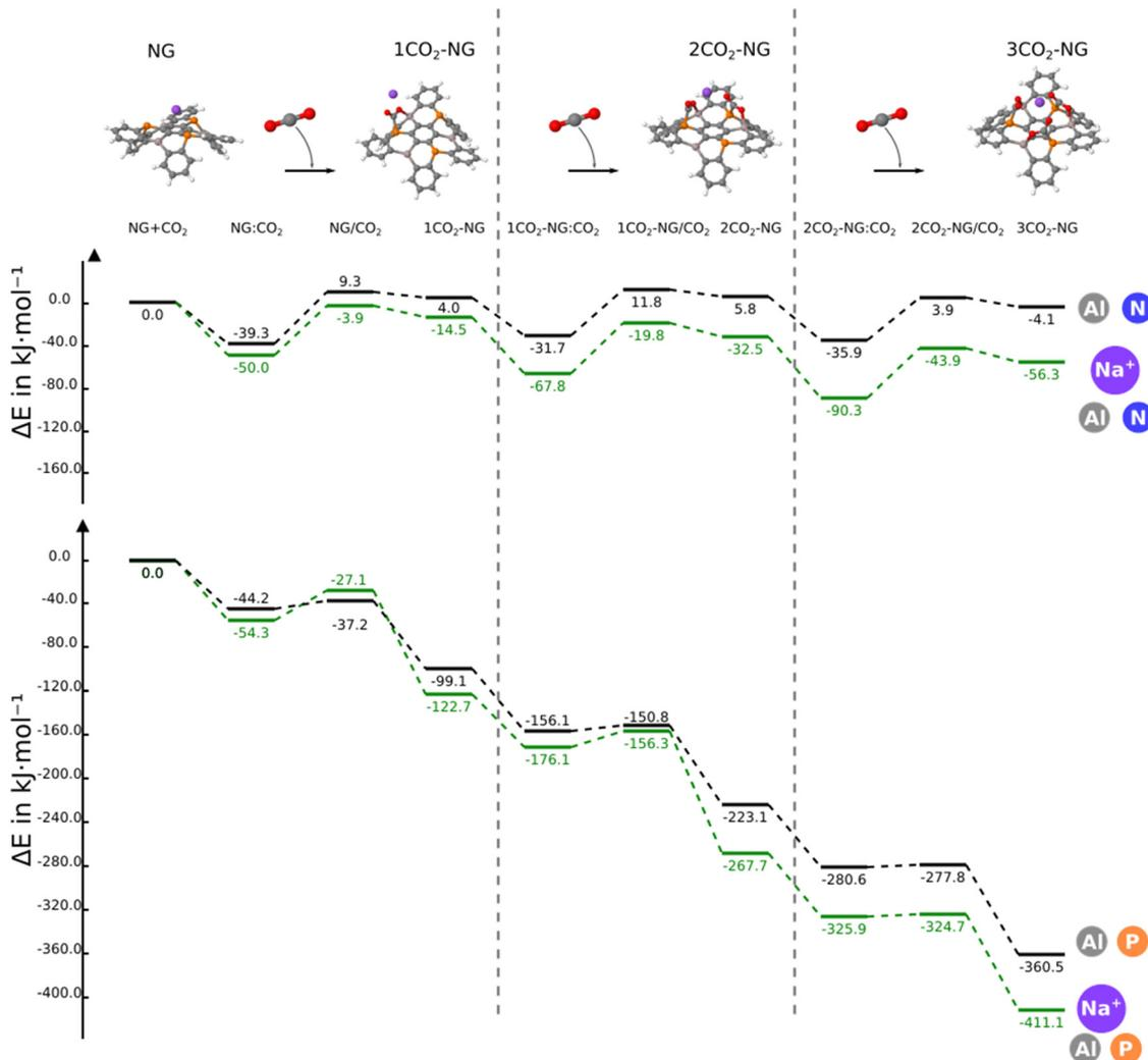
Fig. 8 Comparative energy profiles for the reaction of Al<sub>3</sub>N<sub>3</sub>-NG and Al<sub>3</sub>P<sub>3</sub>-NG in the absence/presence of Na<sup>+</sup> with three CO<sub>2</sub> molecules.
