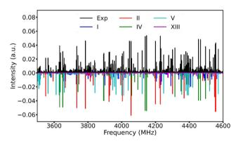
Fig. 2 A section of the experimental broadband rotational spectrum recorded with 1.4 million FIDs with known transitions of the TFB monomer and its rarer isotopologues as well as the TFB  $\cdots$   $H_2O$  adduct removed. The simulated spectra were produced with the experimental rotational constants, the theoretical permanent electric dipole moment components and an estimated rotational temperature of 1 K, as well as their estimated experimental relative abundances.
