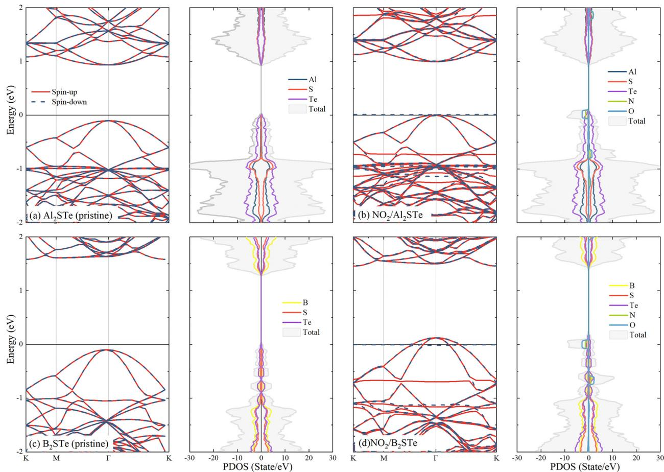
Fig. 4 Display of band structures and partial density of states (PDOS) of molecules adsorbed to  $\text{Al}_2\text{STe}$  and  $\text{B}_2\text{STe}$  materials (using spin-polarized calculations with the Fermi level set to zero).
