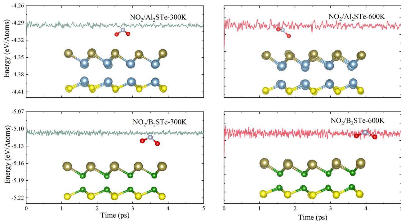
Fig. 3 The energy changes for Al<sub>2</sub>STe and B<sub>2</sub>STe at temperatures of 300 and 600 K, respectively, and side view of the final snapshots obtained from *ab initio* molecular dynamics simulation.
