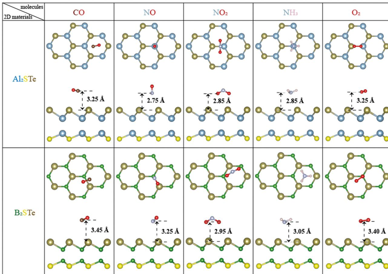
Fig. 1 Optimal adsorption configurations of gas molecules (CO, NO, NO<sub>2</sub>, NH<sub>3</sub>, and O<sub>2</sub>) on Al<sub>2</sub>STe and B<sub>2</sub>STe monolayers, presented from both top and side views.
