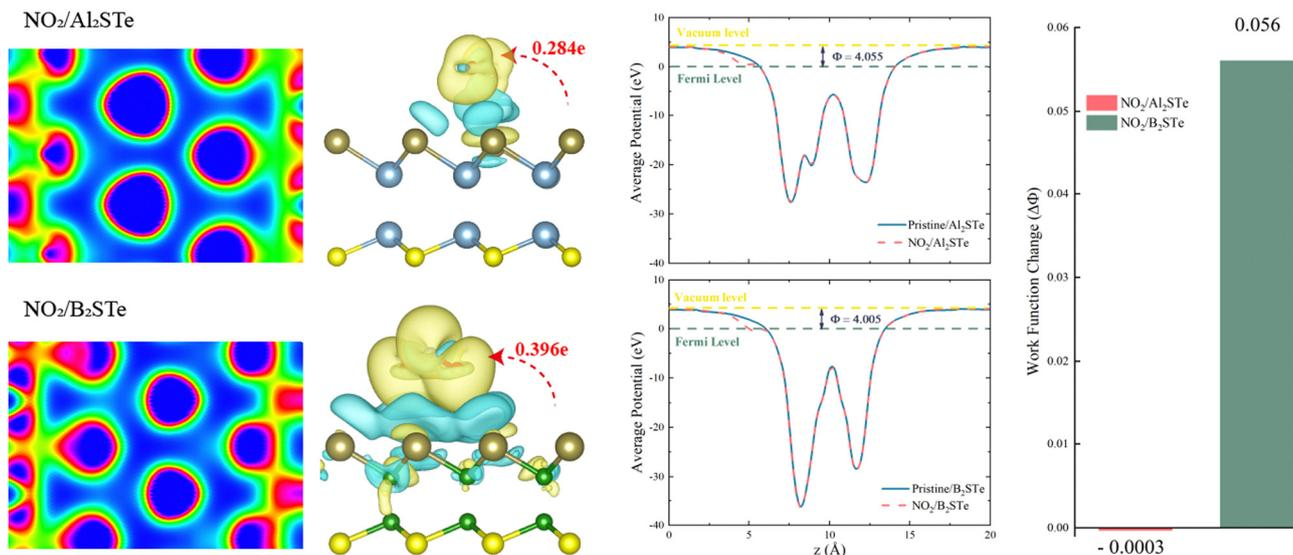
Fig. 5 Electron localization function (ELF), charge density differences, averaged potential, and work function change of  $\text{NO}_2$  gas molecule plots for  $\text{Al}_2\text{STe}$  and  $\text{B}_2\text{STe}$  monolayers. Charge accumulation (depletion) is shown by the yellow (blue) region. The value of the isosurface is calculated as  $5 \times 10^{-4} e \text{ \AA}^{-3}$ . The direction and amount of the charge transfer are also indicated.
