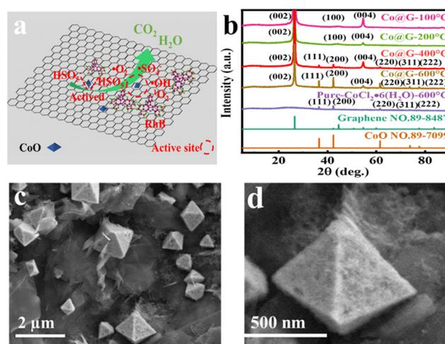
Fig. 1 (a) Schematic illustration of the Fenton-like catalysis mechanism via CoO@graphene. (b) X-ray diffraction (XRD) patterns of CoO@graphene and  $\text{CoCl}_2 \cdot 6\text{H}_2\text{O}$  after calcination at various temperatures up to 600 °C. (c) and (d) The scanning electron microscopy (SEM) image of CoO@graphene and the size of single CoO.
