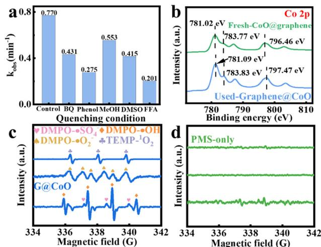
Fig. 3 (a) Pseudo-first order rate constants ( $k_{obs}$ ) from quenching experiments. (b) High resolution spectra of Co 2p for fresh and used CoO@graphene. (c) and (d) EPR spectra of DMPO and TEMP adducts for CoO@graphene/PMS and pure PMS reaction systems.
