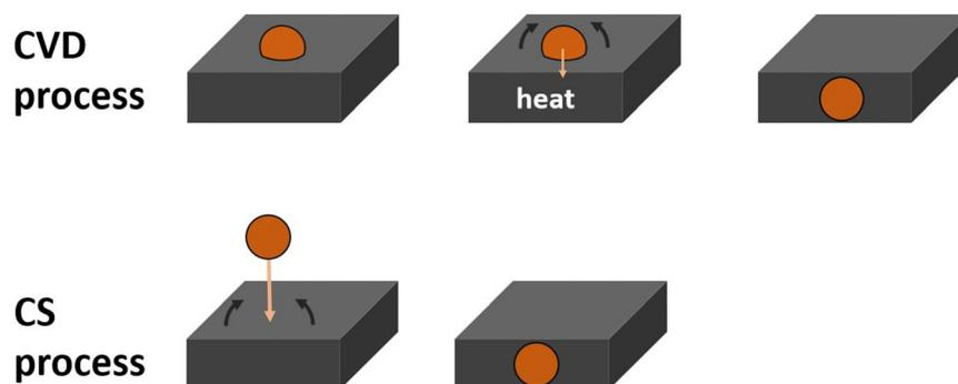
Fig. 5 Schematic of the encapsulation of the Ru clusters for the CVD and CS process. The clusters are shown schematically and do not include the ligands of the Ru<sub>3</sub>(CO)<sub>12</sub> clusters and also do not show a schematic for the growth to larger particles.
