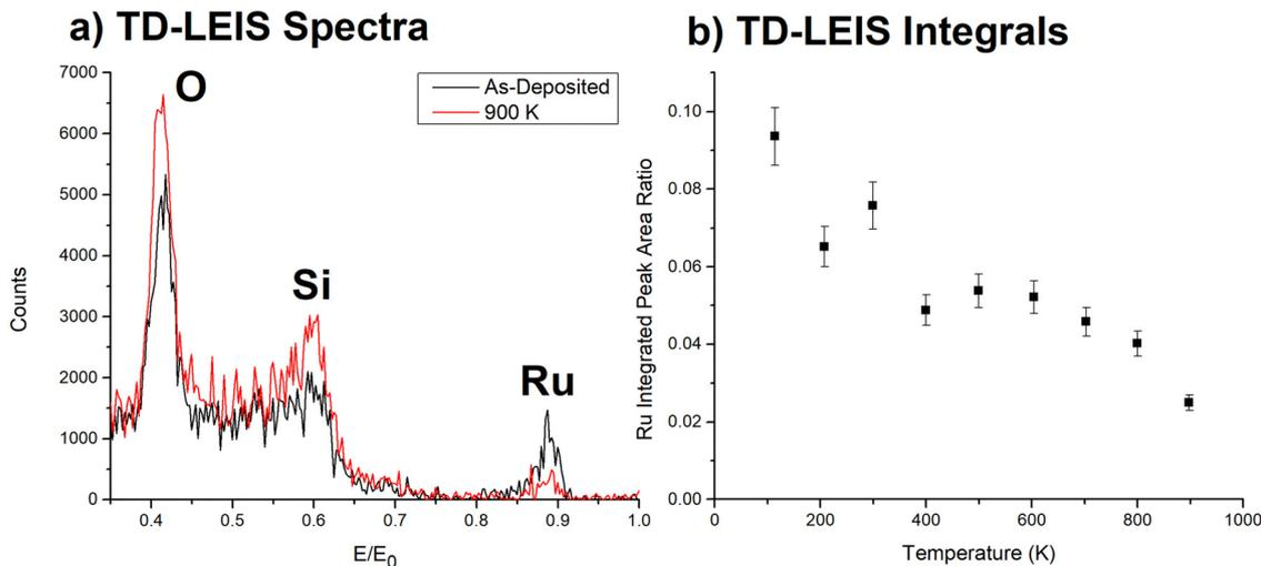
Fig. 2 TD-LEIS of CS-Ru<sub>3</sub>/SiO<sub>2</sub>. (a) LEIS spectra for initial and final temperature measurements. (b) Integrated Ru/(Si + O) peak ratio vs. temperature. Uncertainties in the Ru peak area ratios are ~8%. The sputter effects of the He<sup>+</sup> on the sample are discussed in the ESI† (see Fig. S14).
