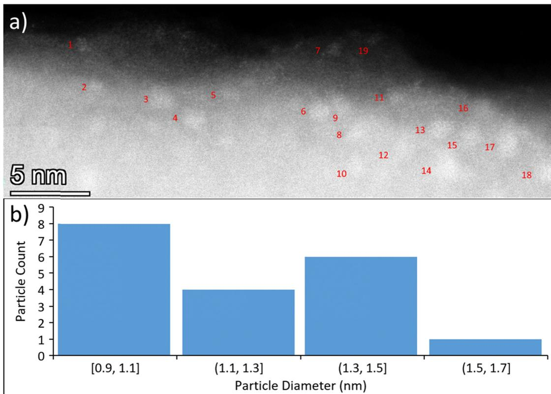
Fig. 4 STEM of CVD-Ru<sub>3</sub>(CO)<sub>12</sub>/HDS-RF-TiO<sub>2</sub>, showing side-on perspective of sample. (a) STEM image with numbered, encapsulated Ru clusters (cluster sizes shown individually in Table S5, ESI<sup>†</sup>). (b) Distribution of particle diameters for encapsulated Ru clusters.
