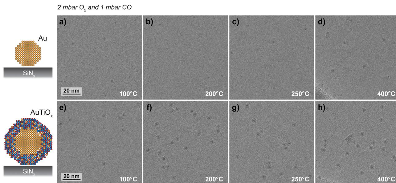
Fig. 7 Behavior of Au and AuTiO<sub>x</sub> nanoparticles under CO oxidation conditions. HRTEM micrographs of Au nanoparticles in (a)–(d) and AuTiO<sub>x</sub> nanoparticles in (e)–(h) acquired *in situ* at the indicated temperatures and during exposure to 1 mbar CO and 2 mbar O<sub>2</sub>. The individual images are cropped from original ones taken at different locations. Image pixel size: 0.037 nm per pixel.
