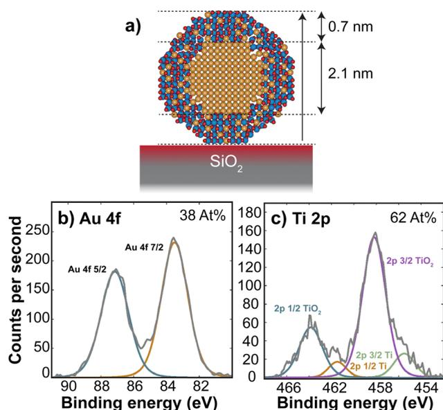
Fig. 3 XPS of the AuTiO<sub>x</sub> nanoparticles on a SiO<sub>2</sub> substrate. (a) Illustration of the estimated thickness of the shell. The XPS signal will arise mainly due to the outermost layers in the shell. (b) Au 4f and (c) Ti 2p peaks in XPS, giving an At% of Au/TiO<sub>2</sub> of 38/62 in the outer shell layers.
