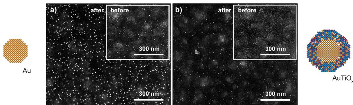
**Fig. 5** Sintering after catalytic testing was observed to be more severe for the Au nanoparticles. SEM images of the (a) Au and (b) AuTiO<sub>x</sub> nanoparticles on the μ-reactors before and after reaction. All SEM images were taken with a TLD secondary electron detector with a beam acceleration voltage of 5 kV. Images pixel size: 0.68 nm (a, before), 0.62 nm (a, after), 0.83 nm (b, before), 0.62 nm (b, after). More images at different magnifications are available in ESI† Section S6.
