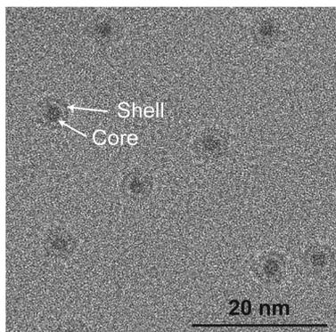
Fig. 2 HRTEM image of AuTiO<sub>x</sub> nanoparticles on SiN<sub>x</sub> chips, after air exposure. The images reveal a core-shell structure with an Au core of size 2.1 ± 0.2 nm. Image pixel size: 0.074 nm per pixel.
