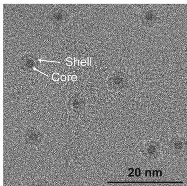
Fig. 2 HRTEM image of AuTiO<sub>x</sub> nanoparticles on SiN<sub>x</sub> chips, after air exposure. The images reveal a core-shell structure with an Au core of size  $2.1 \pm 0.2$  nm. Image pixel size: 0.074 nm per pixel.
