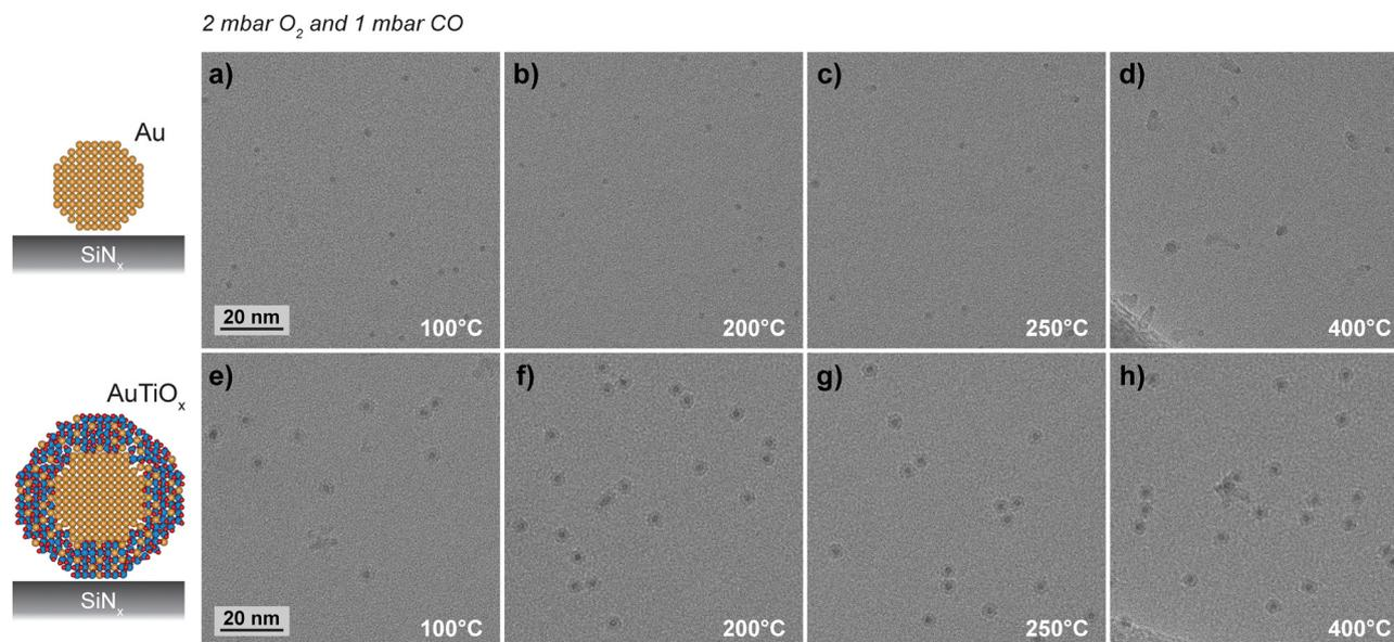
Fig. 7 Behavior of Au and AuTiO<sub>x</sub> nanoparticles under CO oxidation conditions. HRTEM micrographs of Au nanoparticles in (a)–(d) and AuTiO<sub>x</sub> nanoparticles in (e)–(h) acquired *in situ* at the indicated temperatures and during exposure to 1 mbar CO and 2 mbar O<sub>2</sub>. The individual images are cropped from original ones taken at different locations. Image pixel size: 0.037 nm per pixel.
