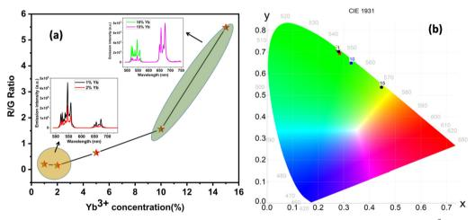
Fig. 8 (a) Variation of red to green emission ratio. Insets show UC spectra in the low and high concentration regions of Yb<sup>3+</sup> sensitizer, and (b) color coordinate diagram depicting variation in CIE values with Yb $^{3+}$  concentrations of ThO<sub>2</sub>:1%Er $^{3+}$ ,X%Yb $^{3+}$  nanophosphor (x = 1, 2, 5, 10 and 15).
