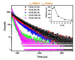
**Fig. 10** UC luminescence decay profile of  $ThO_2:1\%Er^{3+}$ , $x\%Yb^{3+}$  nanophosphor (x=1, 2, 5, 10 and 15). Inset shows the variation in average fluorescence lifetimes with Yb doping.
