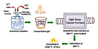
Scheme 1 Schematic showing gel-combustion synthesis of Er<sup>3+</sup>. Yb<sup>3+</sup> co-doped thoria UCNPs.
