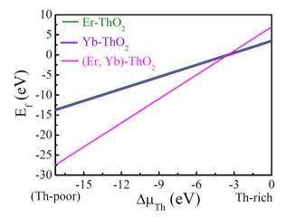
Fig. 3 Variation of defect formation energies for the doped ThO<sub>2</sub>.
