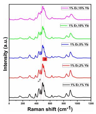
Fig. 5 Raman spectra of ThO<sub>2</sub>:1%Er<sup>3+</sup>,x%Yb<sup>3+</sup> nanophosphor (x = 1, 2, 5,
