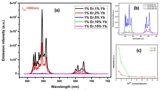
Fig. 7 (a) UC emission spectra, (b) magnified UC spectra of ThO<sub>2</sub>:1%Er<sup>3+</sup>, x%Yb<sup>3+</sup> nanophosphor with x = 5, 10 and 15 and (c) variation of red and green emission intensity with Yb<sup>3+</sup> concentrations, ThO<sub>2</sub>:1%Er<sup>3+</sup>,x%Yb<sup>3+</sup> nanophosphor (x = 1, 2, 5, 10 and 15).
