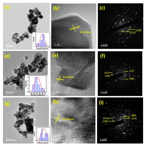
Fig. 4 (a), (d) and (g) TEM images, (b), (e) and (h) HRTEM images and (c), (f) and (i) SAED patterns of ThO<sub>2</sub>:1%Er<sup>3+</sup>,X%Yb<sup>3+</sup> (X = 1, 5 and 15) UCNPs.
