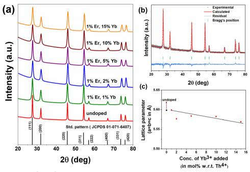
Fig. 1 (a) XRD pattern of  $ThO_2:1\%Er^{3+}$ ,  $x\%Yb^{3+}$  nanophosphor (x = 1, 2, 5, 10 and 15), (b) typical Rietveld fitting of the spectrum, (c) variation of lattice parameters with doping
