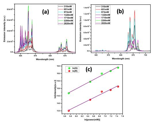
Fig. 9 UC emission spectra of (a) ThO<sub>2</sub>:1%Er<sup>3+</sup>,1%Yb<sup>3+</sup>, (b) ThO<sub>2</sub>:1%Er<sup>3+</sup>,15%Yb<sup>3+</sup> and (c) dependence of pump power on green and red emission in ThO<sub>2</sub>:1%Er<sup>3+</sup>,1%Yb<sup>3+</sup>.
