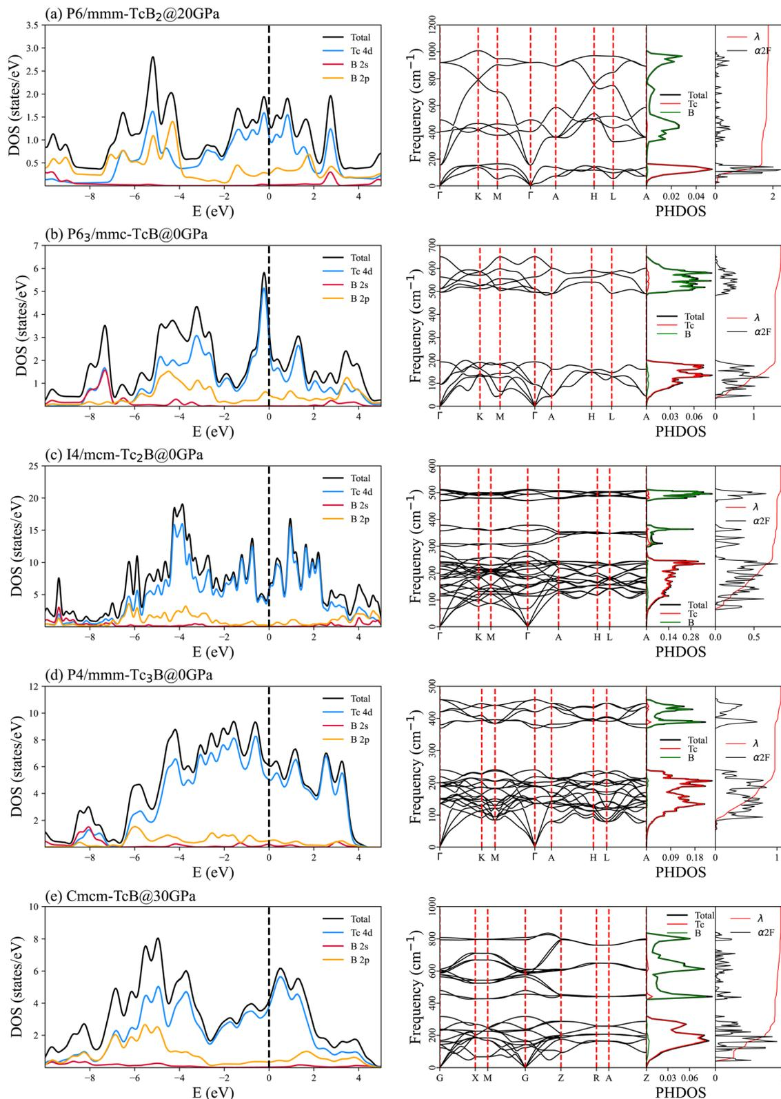
Fig. 4 Total and partial electronic DOS, phonon dispersion relation, phonon density of states (PHDOS), Eliashberg functional  $\alpha^2F(\omega)$  and integrated EPC parameter  $\lambda(\omega)$  of superconducting technetium borides at their lowest dynamically stable pressures. From top to bottom: (a)  $TcB_2$  ( $P6/mmm$ , 20 GPa), (b)  $TcB$  ( $P6_3/mmc$ , 0 GPa), (c)  $Tc_2B$  ( $I4/mcm$ , 0 GPa), (d)  $Tc_3B$  ( $P4/mmm$ , 0 GPa) and (e)  $TcB$  ( $Cmcm$ , 30 GPa).
