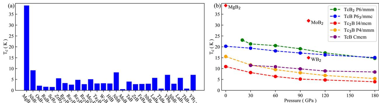
**Fig. 2** (a) Superconducting transition temperatures of metal borides at ambient pressure measured experimentally. (b) Superconducting transition temperatures of TcB<sub>2</sub> (P6/mmm), TcB (P6<sub>3</sub>/mmc), Tc<sub>2</sub>B (I4/mcm), Tc<sub>3</sub>B (P4/mmm) and TcB (Cmcm) as a function of pressure, together with the superconducting transition temperatures of MgB<sub>2</sub> at ambient pressure, and MoB<sub>2</sub> and WB<sub>2</sub> at 100 GPa, measured experimentally (red diamonds).
