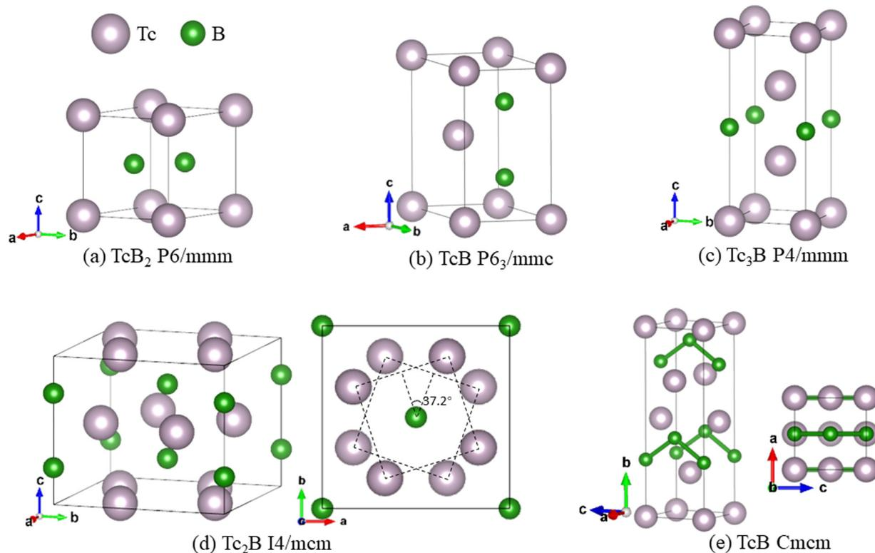
Fig. 3 Crystal structures of superconducting technetium borides. (a)  $\text{TcB}_2$  ( $P6/mmm$ ), (b)  $\text{TcB}$  ( $P6_3/mmc$ ), (c)  $\text{Tc}_3\text{B}$  ( $I4/mcm$ ), (d)  $\text{Tc}_2\text{B}$  ( $P4/mmm$ ) and (e)  $\text{TcB}$  ( $Cmcm$ ). The technetium and boron atoms are represented by spheres of coral and green colors, respectively.
