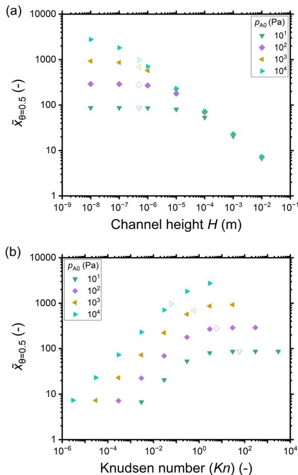
Fig. 5 The penetration depth in terms of the dimensionless distance at half coverage  $\tilde{x}_{\theta=0.5}$  extracted from the saturation profiles shown in Fig. 4 as a function of: (a) the channel height  $H$ , and (b) the Knudsen number. Hollow symbols correspond to the typical PillarHall™ case<sup>17,37</sup> with a 500 nm channel height.
