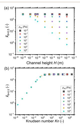
Fig. 8 The penetration depth in terms of the dimensionless distance at half coverage  $\tilde{x}_{\theta=0.5}$  with respect to (a) the channel height H and (b) the Knudsen number. Data was extracted from the saturation profiles shown in Fig. 7. The hollow symbols at 500 nm represent the typical PillarHall™ case.<sup>17,37</sup>
