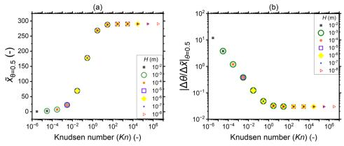
Fig. 10 (a) The penetration depth at half coverage  $\tilde{x}_{\theta=0.5}$  and (b) the absolute value of the slope at half coverage  $|\Delta\theta/\Delta\tilde{x}|_{\theta=0.5}$  plotted as a function of the Knudsen number for a sticking coefficient c of 0.01. The channel heights, reactant partial pressure, and saturation profiles are the same as in Fig. 7. Table 1 lists the other parameters.
