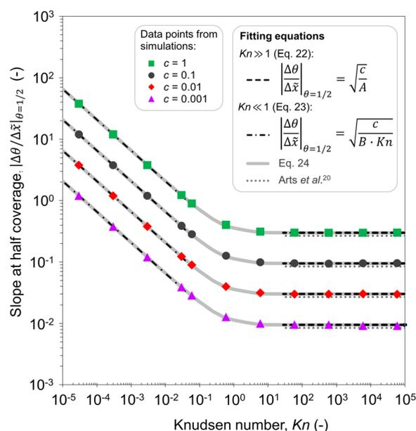
Fig. 12 Fitted data of the absolute value of the slope at half coverage as a function of the Knudsen number. Data points for  $c = 1, 0.1, 0.01$ , and  $0.001$  were obtained using the Ylilammi *et al.*<sup>19</sup> model for diffusion-limited conditions. Fitting parameters of the equations:  $A = 11.1$  and  $B = 23.3$ .
