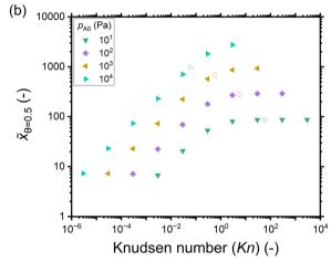
Fig. 5 The penetration depth in terms of the dimensionless distance at half coverage  $\tilde{x}_{\theta=0.5}$  extracted from the saturation profiles shown in Fig. 4 as a function of: (a) the channel height H, and (b) the Knudsen number. Hollow symbols correspond to the typical PillarHall™ case<sup>17,37</sup> with a 500 nm channel height
