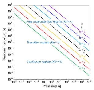
Fig. 2 Knudsen number as a function of pressure at 250 °C, for features with different characteristic limiting sizes "D", calculated from the mean free path (eqn (1) and (2)) for a gas molecule with a hard-sphere diameter of  $6 \times 10^{-10}$  m.
