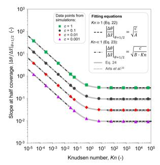
Fig. 12 Fitted data of the absolute value of the slope at half coverage as a function of the Knudsen number. Data points for c = 1, 0.1, 0.01, and 0.001 were obtained using the Ylilammi et al. 19 model for diffusion-limited conditions. Fitting parameters of the equations: A = 11.1 and B = 23.3.
