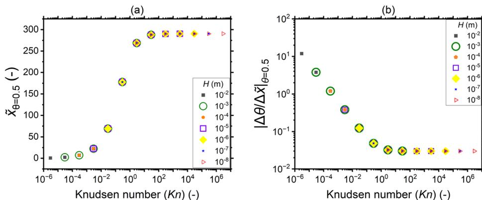
Fig. 10 (a) The penetration depth at half coverage  $\bar{X}_{\theta=0.5}$  and (b) the absolute value of the slope at half coverage  $|\Delta\theta/\Delta\bar{x}|_{\theta=0.5}$  plotted as a function of the Knudsen number for a sticking coefficient  $c$  of 0.01. The channel heights, reactant partial pressure, and saturation profiles are the same as in Fig. 7. Table 1 lists the other parameters.
