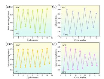
Fig. 5 Temperature-dependent reversibility of a thin-film temperature detector for CdSe/ZnS with a shell thickness of (a) 0 ML, (b) 1 ML, (c) 4 MLs, and (d) 7 MLs.
