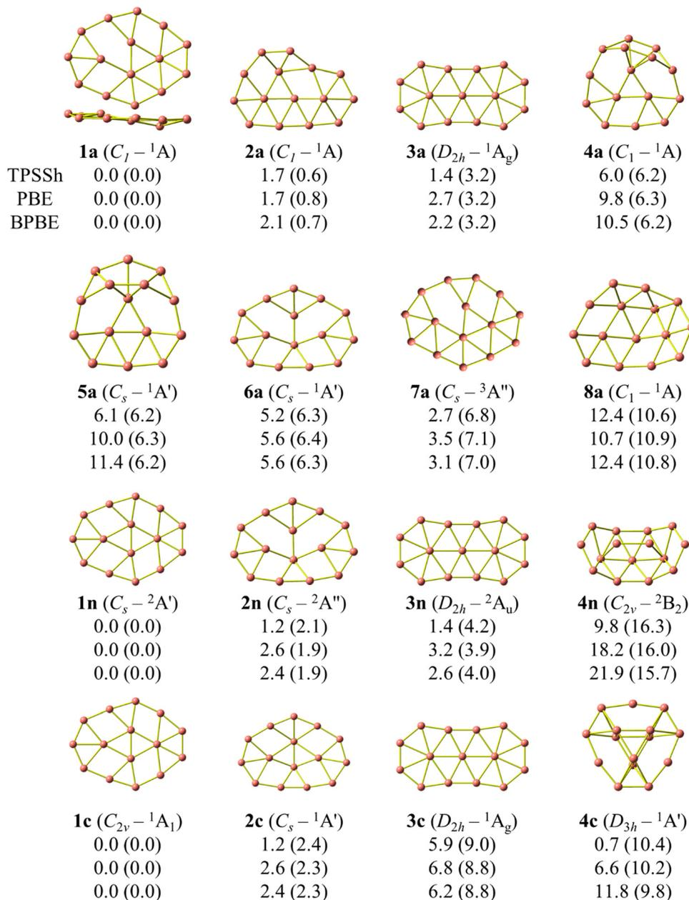
**Fig. 1** Optimized geometries of  $B_{15}^{+/0/-}$  using TPSSh, PBE and BPBE functionals with the 6-311+G(d) basis set with symmetry point group and electronic state. Relative energies ( $\text{kcal mol}^{-1}$ ) are obtained with ZPE corrections without scaling at the respective functional, TPSSh (upper values), PBE (middle) and BPBE (lower). Relative energies obtained by single-point (U)CCSD(T)/aug-cc-pVTZ energies at corresponding DFT geometries and ZPE corrections are given in parentheses.
