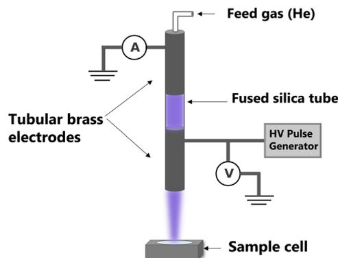
Scheme 2 Scheme of a LTP's set-up.
