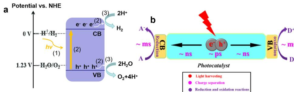
Fig. 1 Photocatalytic H<sub>2</sub> evolution process (a). The kinetic times for separation, transfer, and reaction of photogenerated charge carriers (b). Reproduced with permission from ref. 31. Copyright 2021, Wiley-VCH.
