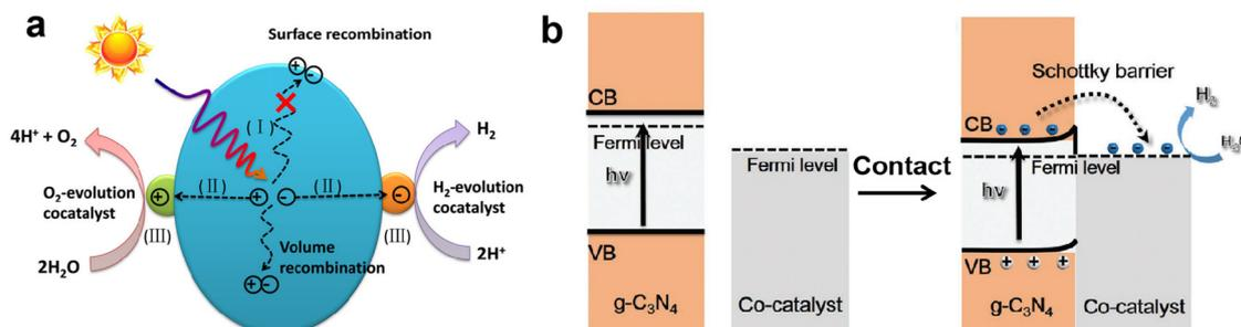
Fig. 10 The role of cocatalyst in photocatalytic water splitting (a). Reproduced with permission from ref. 139. Copyright 2020, Wiley-VCH. The band alignment between metallic cocatalysts and n-type  $g\text{-C}_3\text{N}_4$  after intimate contact (b). Reproduced with permission from ref. 140. Copyright 2021, Wiley-VCH.
