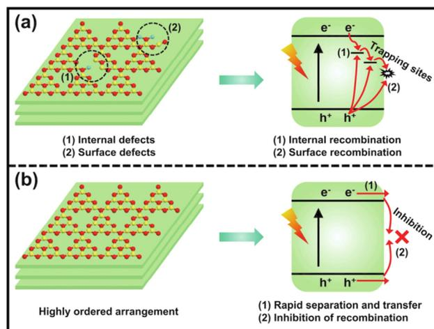
Fig. 2 The charge separation and transfer of conventional poorly-crystalline g-C<sub>3</sub>N<sub>4</sub> (a) and highly ordered g-C<sub>3</sub>N<sub>4</sub> (b). Reproduced with permission from ref. 39. Copyright 2023, Elsevier.
