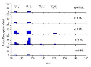
Fig. 2 (top) Anion desorption yield of clusters and/or molecular anions heavier than benzene from 2ML of benzene deposited on a Pt surface irradiated at different electron impact energies. (bottom) Anion desorption yield of different benzene layer thicknesses deposited on a Pt surface irradiated at 950 eV electron impact energy.
