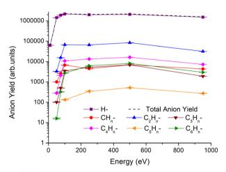
Fig. 1 (top) Electron stimulated desorption yields of anionic fragments for different thicknesses of benzene deposited on a Pt surface irradiated at an electron impact energy of 950 eV. (bottom) Electron stimulated desorption yields of anionic fragments from 2ML of benzene deposited on a Pt surface irradiated at different electron impact energies.
