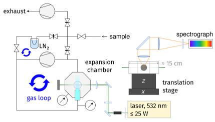
Fig. 1 Sketch of the cookie-jet setup. Top-view on the left side, side-view on the right side.
