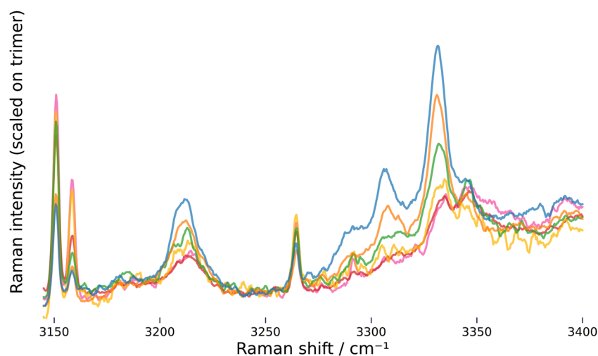
Fig. 3 High resolution Raman spectra, zoomed in on tetramer, pentamer and overtone band. Ro-vibrational lines of the monomer were removed from the overtone band and a moving average filter weighted by a Gaussian window ( \sigma = 1.5 \text{ cm}^{-1} ) was applied. The same color code as in Fig. 2 applies.
