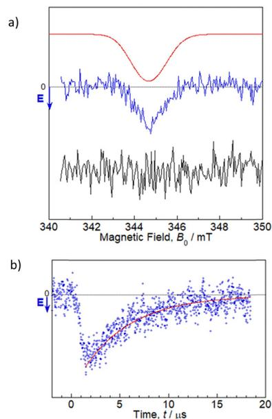
Fig. 2 TREPR spectra for a 100  $\mu\text{M}$  MeCN solution of **1** at 298 K. Microwave power: 2.1 mW. (a) Spectrum at a delay of 2  $\mu\text{s}$  after the laser pulse (blue), simulation spectrum using the parameters described in the text (red), and a comparison with FlH-MB (black) as a reference. (b) Transient signal at  $B = 344.8$  mT (blue) and exponential fitting (red). Details of the fitting are described in the text.
