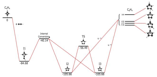
Fig. 2 Reaction pathway for the formation of benzvalyne via  $C_2H$  addition to  $c-C_4H_4$  in kcal  $mol^{-1}$ . Internal conversion<sub>a</sub> represents the intersection seen in Fig. 3.
