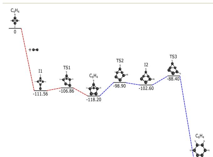
Fig. 1 Reaction pathway for the formation of c- $C_6H_4$  via  $C_2$  addition to c- $C_4H_4$  in kcal mol<sup>-1</sup>. Red dashed lines represent this research, and blue dashed lines from Poland et al. 12
