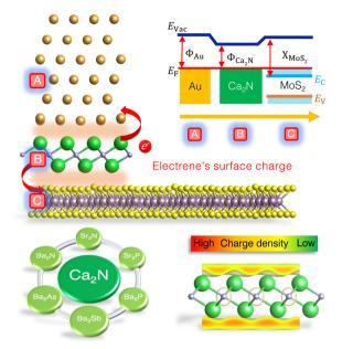
Fig. 1 Top: Schematic design of the Au/MoS<sub>2</sub> interface with monolayer Ca<sub>2</sub>N as an intermediate layer. The associated band diagram indicates the removal of the Schottky barrier upon metallization of the MoS<sub>2</sub> bands. Bottom: List of all stable M2X electrides, along with a 3D representation of the electrene's surface charge.
