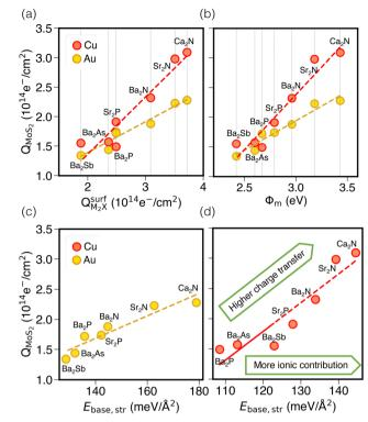
Fig. 3 (a) Correlation of  $Q_{\text{MoS}_2}$  and  $Q_{\text{M}_2\text{X}}^{\text{surf}}$  in Au and Cu-based interfaces. (b) Correlation of  $Q_{MoS_2}$  and the monolayer electrene work function ( $\Phi_m$ ). Also shown are correlations between the base-functional (ionic) component of the exfoliation energy and  $Q_{MoS_{\eta}}$  for Au (c) and Cu (d) interfaces, respectively.
