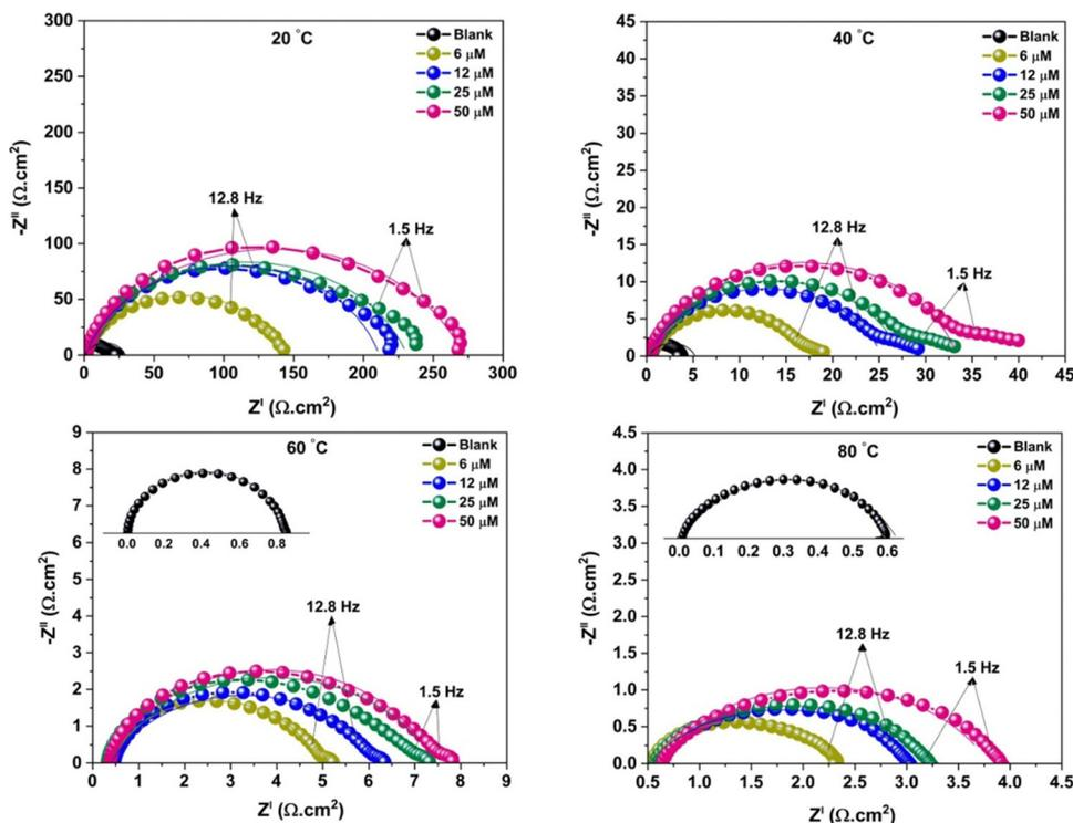
Fig. 8 Nyquist graphs for MS in the 15% HCl medium, with and without different CHEC concentrations at 20 °C, 40 °C, 60 °C, and 80 °C<sup>65</sup> [Reproduced from ref. 65 with permission; Copyright@Elsevier; 2021].
