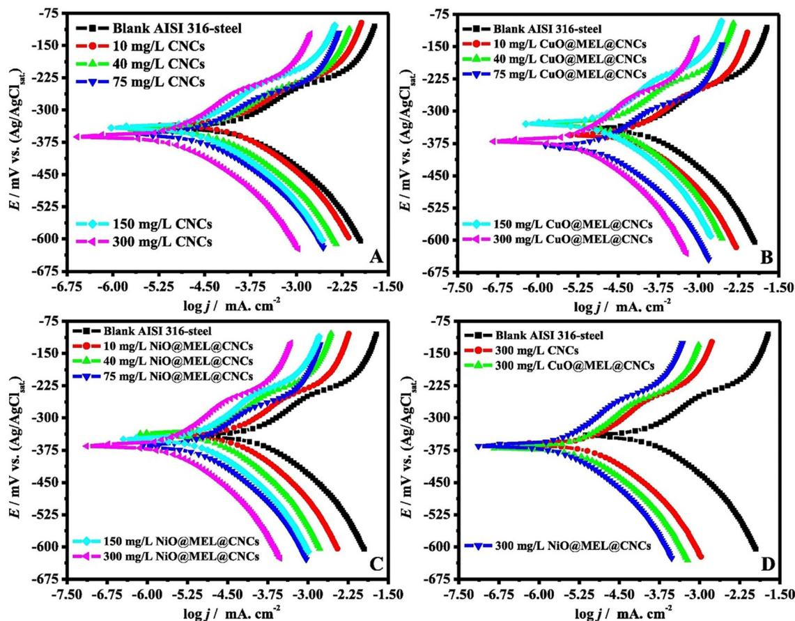
Fig. 11 PDP curves for AISI360-steel measured in 1.0 M  $\text{H}_2\text{SO}_4$  solution with and without (blank) varying concentrations of (A) CNC, (B)  $\text{CuO@MEL@CNCs}$  and (C)  $\text{NiO@MEL@CNCs}$ , and (D) with 300 ppm of different nanocomposites present<sup>133</sup> [Reproduced from ref. 133 with permission; Copyright@Elsevier; 2021].
