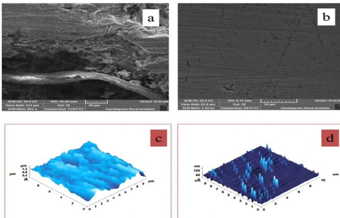
Fig. 6 (i) SEM and (ii) AFM pictures of mild steel specimens that are (a, c) uninhibited and (b, d) inhibited by AHEC<sup>101</sup> [Reproduced from ref. 101 with permission; Copyright@Elsevier; 2016].
