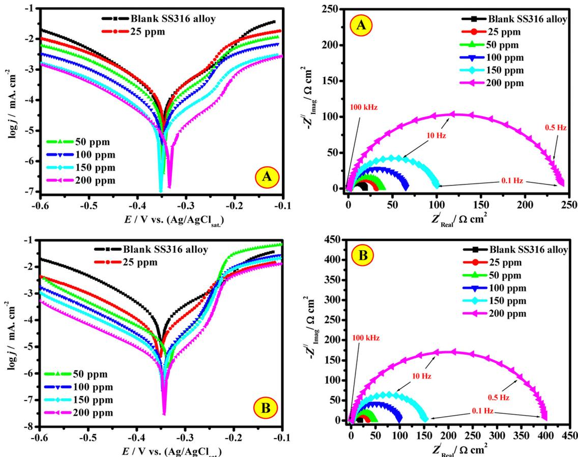
Fig. 13 PDP (left side) Nyquist (right side) diagrams of the SS316 alloy at  $T = 323$  K in 2.0 M HCl with and without different concentrations of (A) CEL and (B) NCC<sup>134</sup> [Reproduced from ref. 134; open access publication, copyright permission not required].
