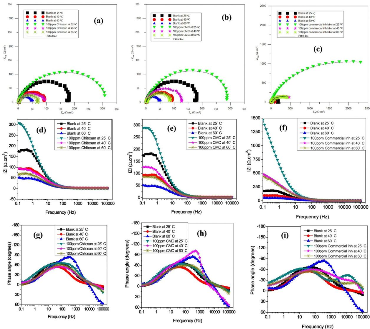
Fig. 10 API 5L X60 steel impedance plots in a  $\text{CO}_2$ -saturated 3.5% NaCl solution with and without 100 ppm of commercial inhibitor, chitosan, and CMC at different temperatures represented by (a–c) Nyquist, (d–f) Bode frequency, and (g–i) Bode phase angle representations<sup>115</sup> [Reproduced from ref. 115 with permission; Copyright@Elsevier, 2018].
