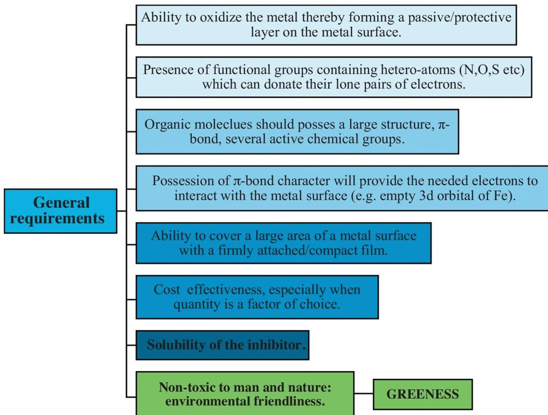
Fig. 5 Schematic presentation of the general requirements of a compound to be used as a corrosion inhibitor (left side)<sup>29</sup> [Reproduced from ref. 29 with permission; Copyright@Elsevier; 2016].
