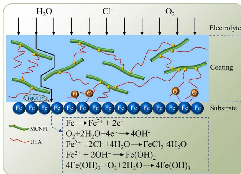
Fig. 15 Diagrammatic illustration of the MCNFI/UEA composite coatings' corrosion resistance mechanism on tinplate substrates<sup>150</sup> [Reproduced from ref. 150 with permission; Copyright@Elsevier; 2022].
