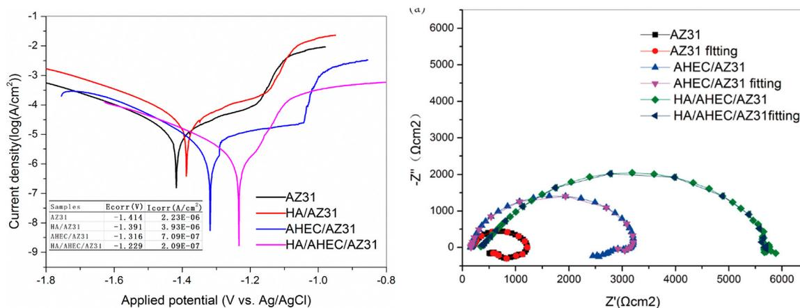
Fig. 14 The polarization (left side) and Nyquist (right side) plots for AZ31 corrosion in simulated body fluid with and without HA, AHEC and HA/AHEC coatings<sup>145</sup> [Reproduced from ref. 145; open access publication, copyright permission not required].
