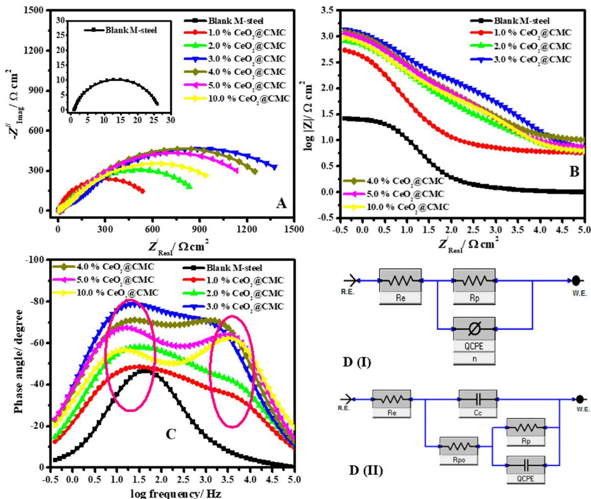
Fig. 16 Nyquist (A), Bode (B), and Bode phase (C) plots in 1.0 M HCl solution for MS and coated with different percentages of CeO<sub>2</sub>-CMC at 50 °C, and (D) EEC for systems that are uncoated (D(II)) and coated (D(I))<sup>151</sup> [Reproduced from ref. 151; open access publication, copyright permission not required].
