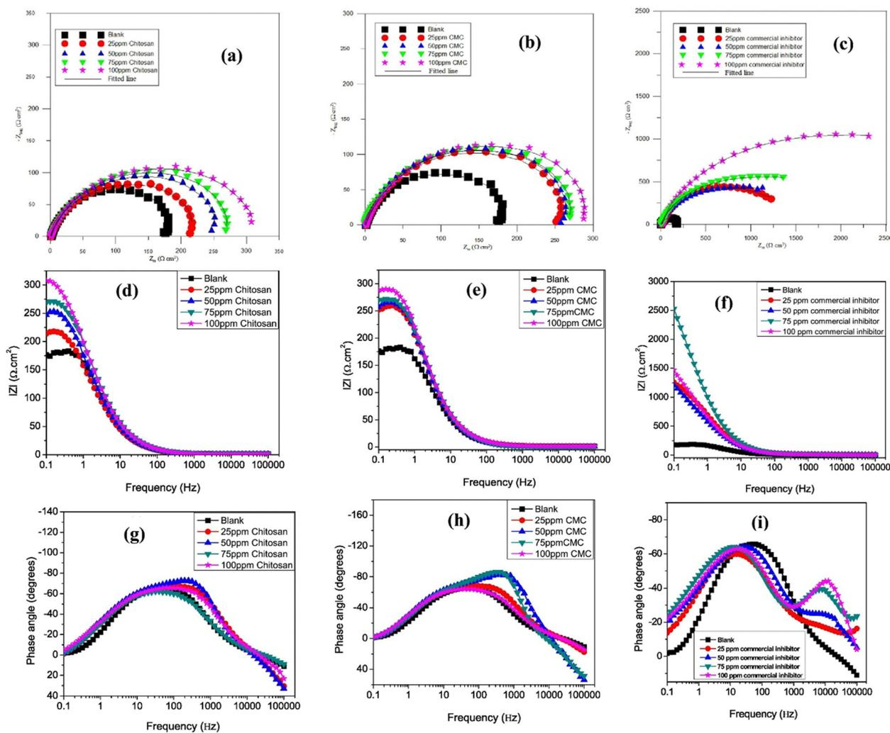
Fig. 9 API 5L X60 steel impedance plots in a  $\text{CO}_2$ -saturated 3.5% NaCl solution with and without different commercial inhibitors, chitosan, and CMC concentrations in (a–c) Nyquist, (d–f) Bode frequency, and (g–i) Bode phase angle representations at  $25^\circ\text{C}$ <sup>115</sup> [Reproduced from ref. 115 with permission; Copyright@Elsevier; 2018].
