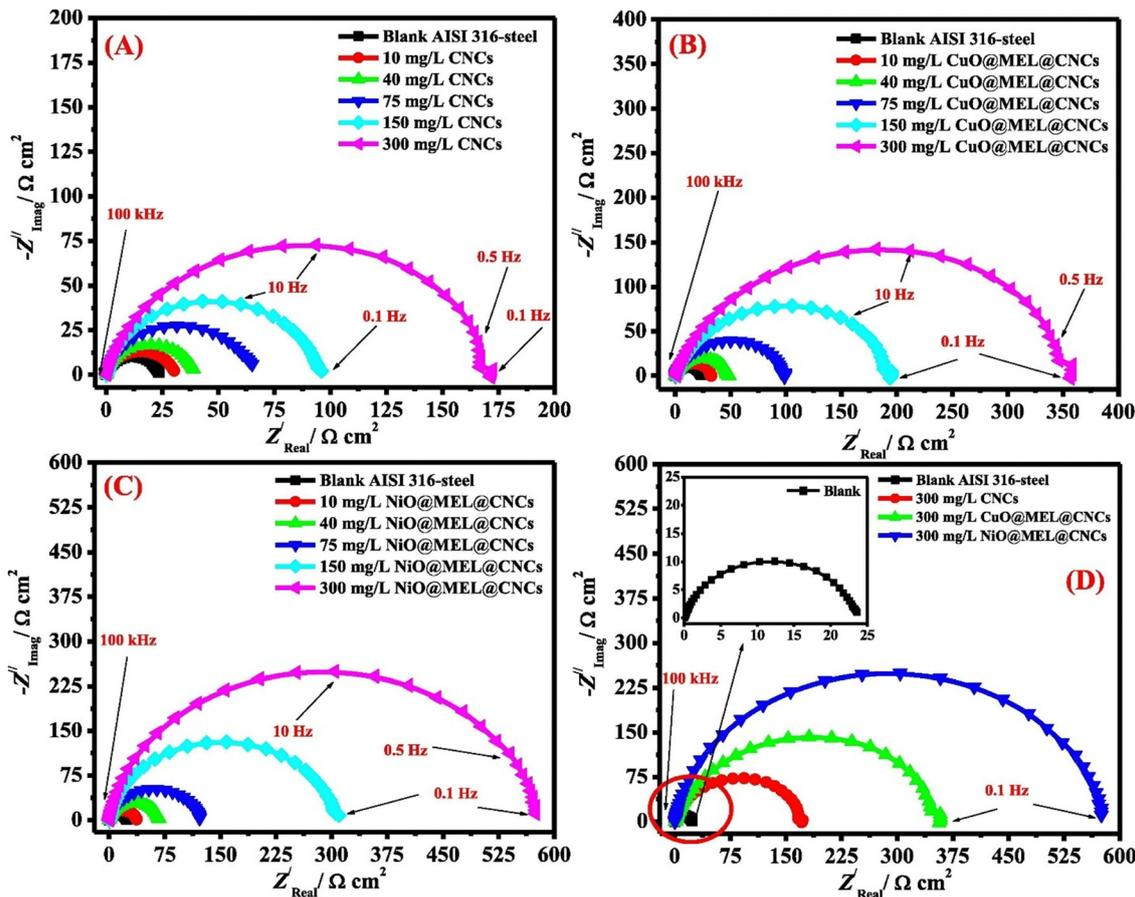
Fig. 12 Nyquist curves for AISI360-steel measured in 1.0 M  $\text{H}_2\text{SO}_4$  solution with and without (blank) varying concentrations of (A) CNC, (B)  $\text{CuO@MEL@CNCs}$  and (C)  $\text{NiO@MEL@CNCs}$ , and (D) with 300 ppm of different nanocomposites present<sup>133</sup> [Reproduced from ref. 133 with permission; Copyright@Elsevier; 2021].
