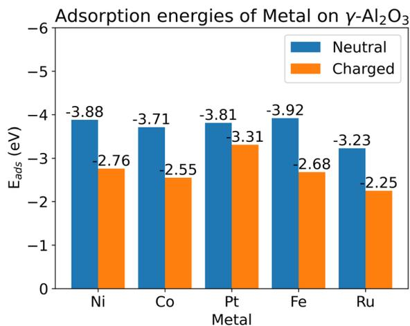
Fig. 4 Adsorption energies of metal atoms on  $\gamma\text{-Al}_2\text{O}_3$  support with and without surface charging.
