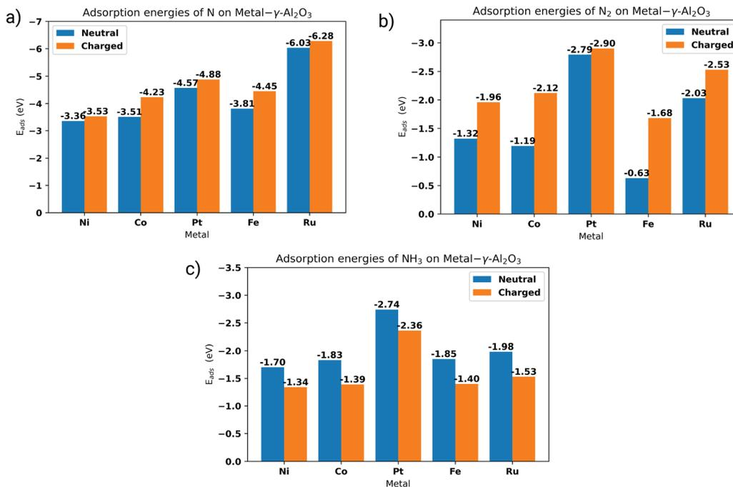
Fig. 5 (a) N, (b) N<sub>2</sub>, and (c) NH<sub>3</sub> adsorption energies on neutral (blue bars) and charged (orange bars) M- $\gamma$ -Al<sub>2</sub>O<sub>3</sub>. M indicates different single metal atoms as specified on the x-axis.
