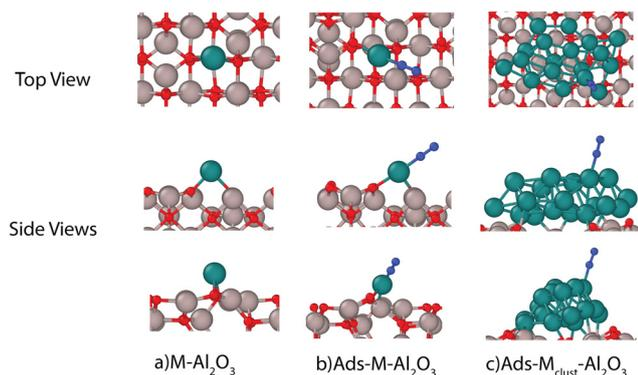
Fig. 3 Typical adsorption geometries obtained using DFT calculations with (a) metal (M: Ru) on support ( $\text{Al}_2\text{O}_3$ ), (b)  $\text{N}_2$  as adsorbate (Ads) with metal atom on support, and (c)  $\text{N}_2$  as adsorbate with metal cluster on support (atom colors: red-oxygen, blue-nitrogen, green-ruthenium, and gray: aluminum).
