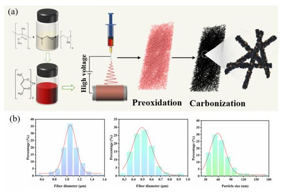
Fig. 1 (a) Schematic illustration of the preparation process of  $Fe@Fe_2O_3/PCNFs$ . (b) Fiber diameter and distribution curves: PAN/PMMA/FeAcAc electrospun nanofibers,  $Fe@Fe_2O_3/PCNFs$ , and  $Fe@Fe_2O_3$  nanoparticles.
