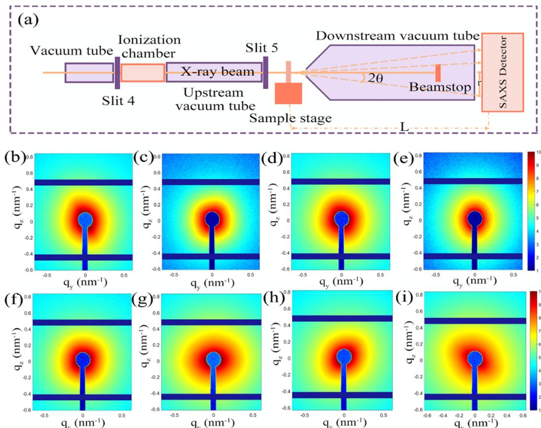
Fig. 5 (a) Schematic diagram of beam line terminal device. The SAXS patterns of the composites with different potentials: (b) initial, (c) discharge to 1.5 V, (d) discharge to 1.0 V, (e) discharge to 0.5 V, (f) discharge to 0.01 V, (g) charge to 1.0 V, (h) charge to 1.5 V, and (i) charge to 3.0 V.
