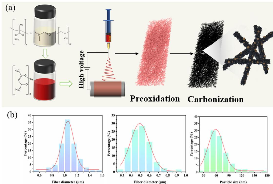
Fig. 1 (a) Schematic illustration of the preparation process of Fe@Fe<sub>2</sub>O<sub>3</sub>/PCNFs. (b) Fiber diameter and distribution curves: PAN/PMMA/FeAcAc electrospun nanofibers, Fe@Fe<sub>2</sub>O<sub>3</sub>/PCNFs, and Fe@Fe<sub>2</sub>O<sub>3</sub> nanoparticles.
