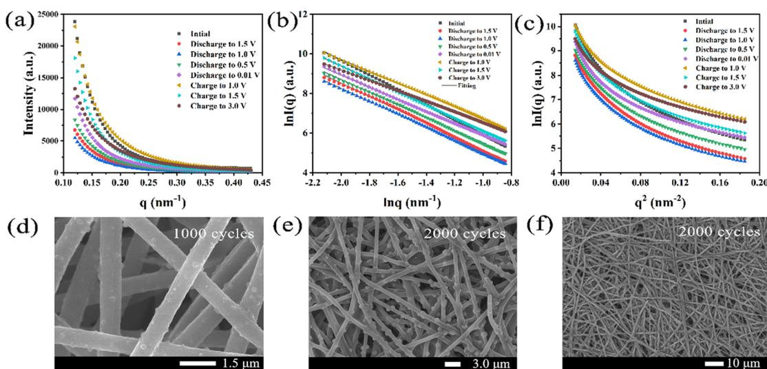
Fig. 6 (a) Curves of intensity ( $I$ ) and scattering vector ( $q$ ) under different charge–discharge potentials. (b) Curves of  $\ln I$  and  $\ln q$  under different charge–discharge potentials. (c) Curves of  $\ln I$  and  $q^2$  under different charge–discharge potentials. SEM images of the electrode plate after cycling: (d) 1000 cycles, (e) 2000 cycles, and (f) 2000 cycles.
