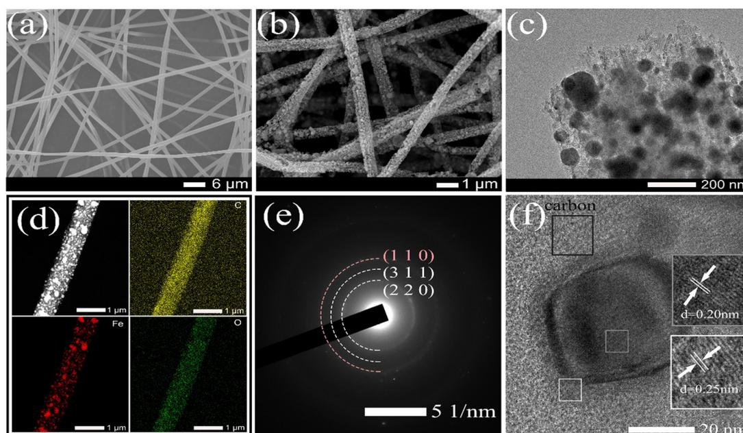
Fig. 2 (a) SEM image of pristine PAN/PMMA/FeAcAc electrospun nanofibers. (b) SEM image of Fe@Fe<sub>2</sub>O<sub>3</sub>/PCNFs. (c) Low-resolution TEM image of Fe@Fe<sub>2</sub>O<sub>3</sub>/PCNFs. (d) Results of EDS elemental mapping of Fe@Fe<sub>2</sub>O<sub>3</sub>/PCNFs corresponding to C, Fe, and O. (e) Selected area electron diffraction (SAED) pattern of Fe@Fe<sub>2</sub>O<sub>3</sub>/PCNFs. (f) HRTEM image of Fe@Fe<sub>2</sub>O<sub>3</sub>/PCNFs.
