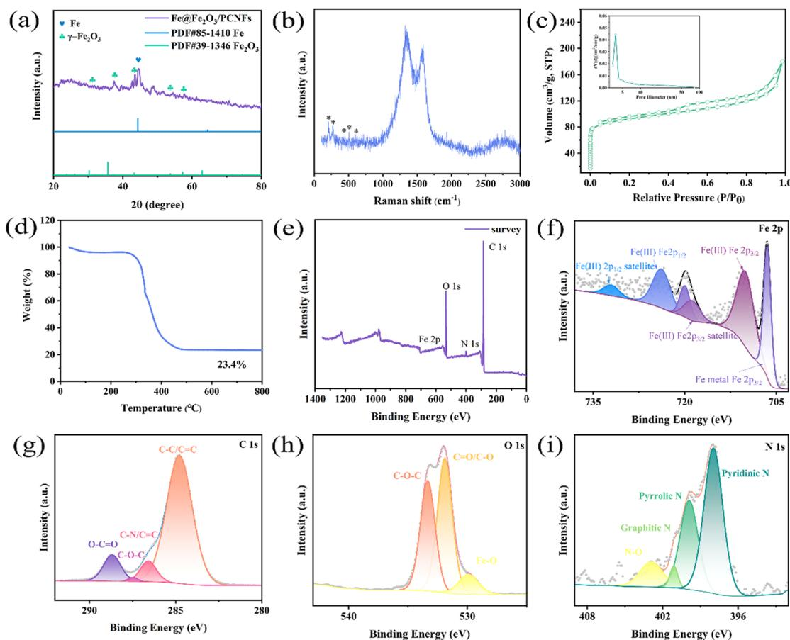
Fig. 3 (a) XRD pattern, (b) Raman spectra, (c) N<sub>2</sub> adsorption/desorption isotherm curve, and pore size distribution diagram (illustration). (d) The results of TGA. XPS spectra: (e) survey, (f) Fe 2p spectrum, (g) C 1s spectrum, (h) O 1s spectrum, and (i) N 1s spectrum of Fe@Fe<sub>2</sub>O<sub>3</sub>/PCNFs.
