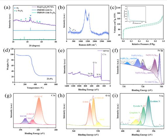
Fig. 3 (a) XRD pattern, (b) Raman spectra, (c) N2 adsorption/desorption isotherm curve, and pore size distribution diagram (illustration). (d) The results of TGA. XPS spectra: (e) survey, (f) Fe 2p spectrum, (g) C 1s spectrum, (h) O 1s spectrum, and (i) N 1s spectrum of Fe@Fe<sub>2</sub>O<sub>3</sub>/PCNFs.
