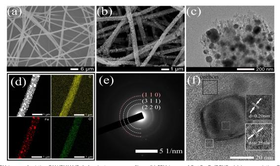
Fig. 2 (a) SEM image of pristine PAN/PMMA/FeAcAc electrospun nanofibers. (b) SEM image of Fe@Fe $_2O_3$ /PCNFs. (c) Low-resolution TEM image of Fe@Fe $_2O_3$ /PCNFs. (d) Results of EDS elemental mapping of Fe@Fe $_2O_3$ /PCNFs corresponding to C, Fe, and O. (e) Selected area electron diffraction (SAED) pattern of Fe@Fe $_2O_3$ /PCNFs. (f) HRTEM image of Fe@Fe $_2O_3$ /PCNFs.
